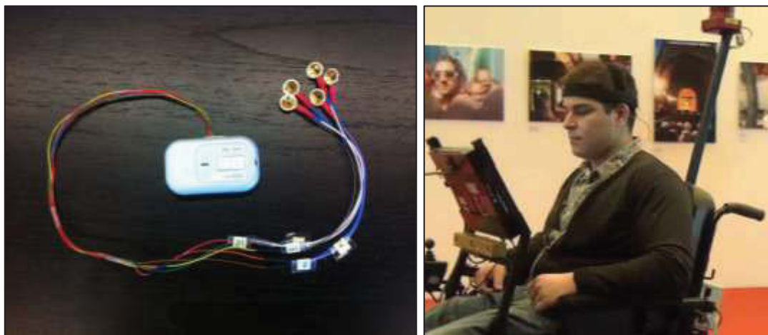
Figure 5-12: „Aviator“ EEG Device Prototype Developed at UTS; User Wearing the Prototype
