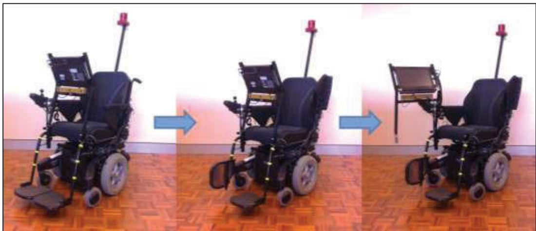
Figure 5-8: TIM Final Stage Prototype Opening Design
