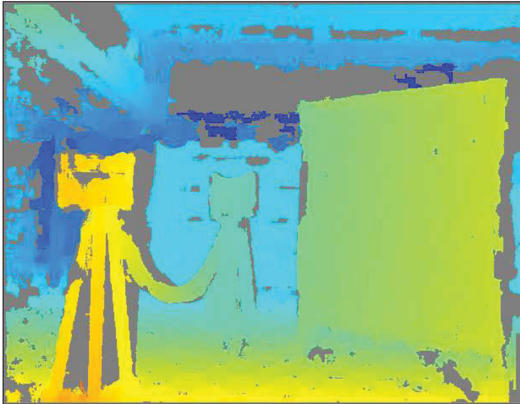
Figure 3-13: Produced Disparity Image of Example Scene Setup
