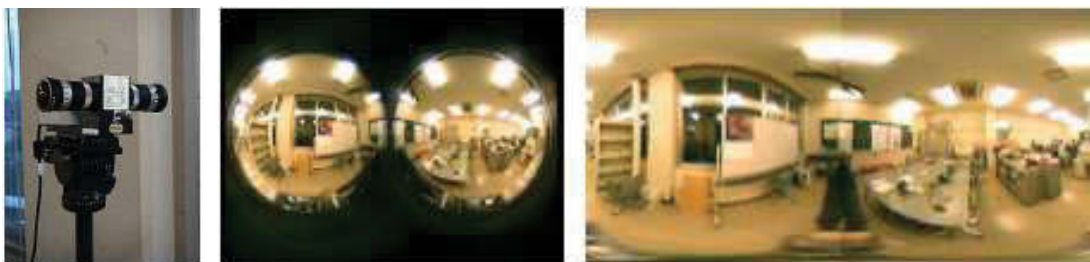
Figure 2-32: Spherical camera; images captured; panoramic conversion (Li & Isago 2007)
