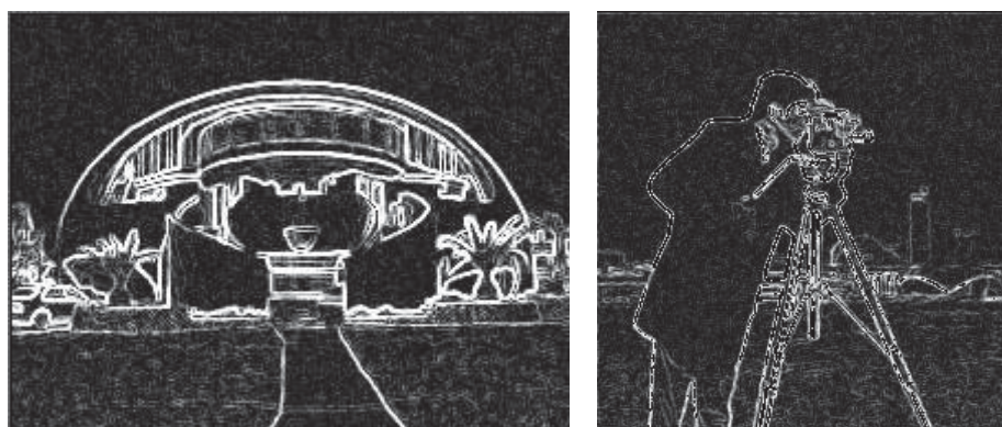
Figure 4-36: Edge Detection Example: Traditional Prewitt Edge Detection (Yang et al. 2011)
