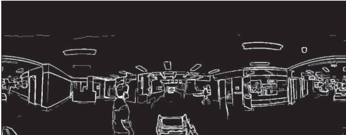
Figure 4-38: Advanced Obstacle Detection Processing: Improved Prewitt Edge Detection
