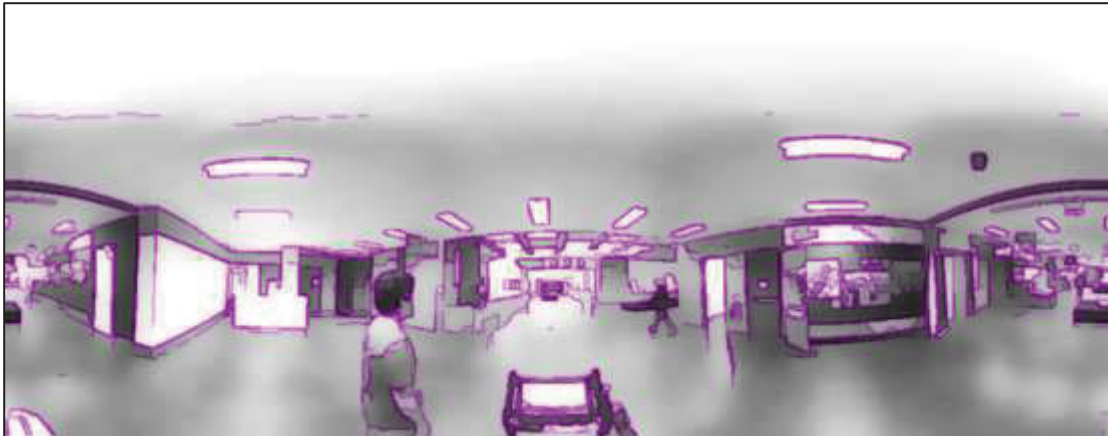
Figure 4-40: Advanced Obstacle Detection Processing: Edge Overlay on Smoothed Grey-scale Image
