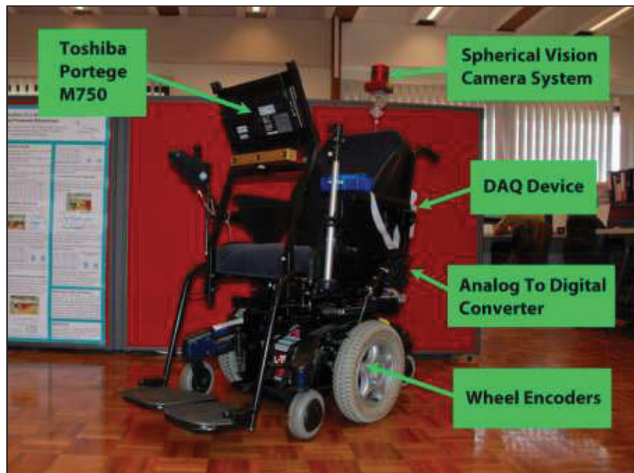
Figure 4-4: TIM Stage 2 Prototype: Integrated Wheelchair Hardware with Spherical Vision Cameras
