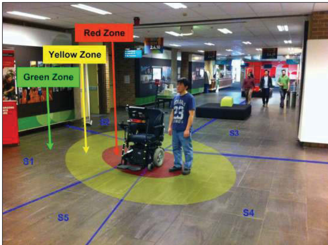
Figure 4-17: „Traffic Light“ Zones and Vision Range Segmentation Photo Display
