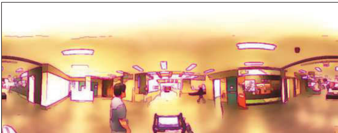
Figure 4-39: Advanced Obstacle Detection Processing: Edge Overlay on Smoothed Colour Image
