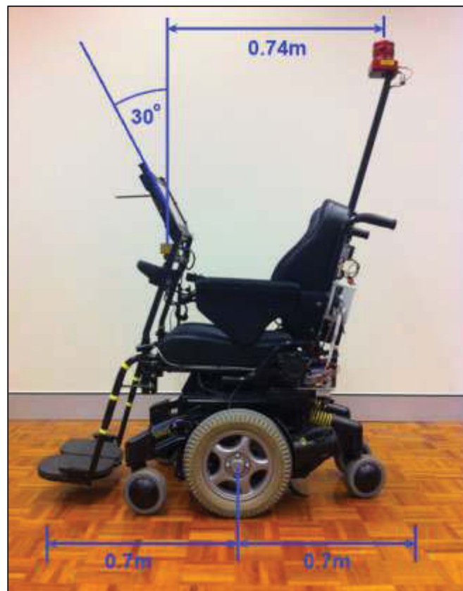
Figure 5-6: TIM Final Stage Prototype Hardware Dimensional Measurements: Side View
