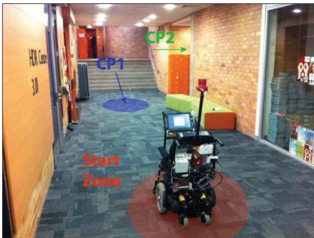
Figure 5-17: „Static Course“ Experimental Study Setup: TIM Smart Wheelchair at the Start Zone
