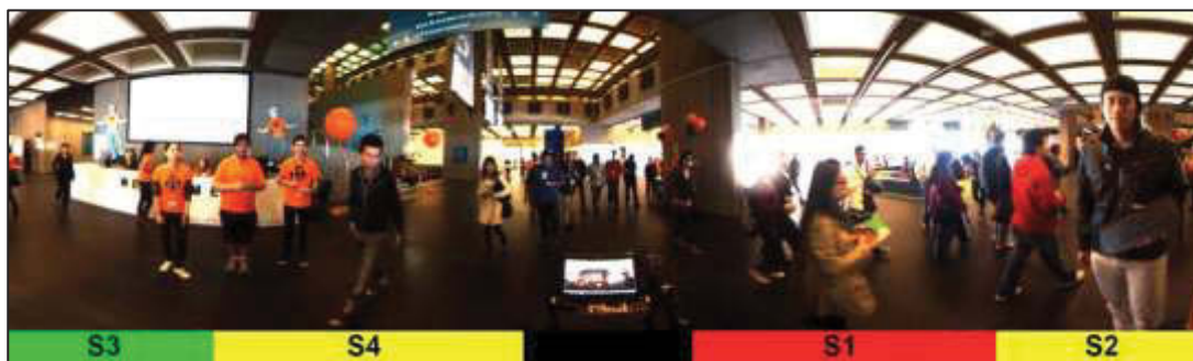
Figure 4-48: User Interface Visual Panoramic Video Feed with Real-time „Traffic Light“ Zone Results
