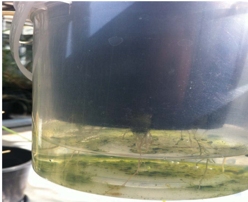
Figure 3-13 The regenerated roots, grow and cross the 'nylon gauze' into the water environment. The 'green' parts are root exudates. Once the newly regenerated roots come into the groundwater, the plant will actively take up metals.
