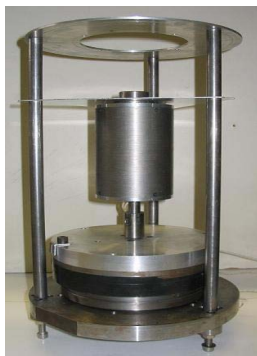
Figure 11. Cogging torque test set-up of the claw pole SMC motor
