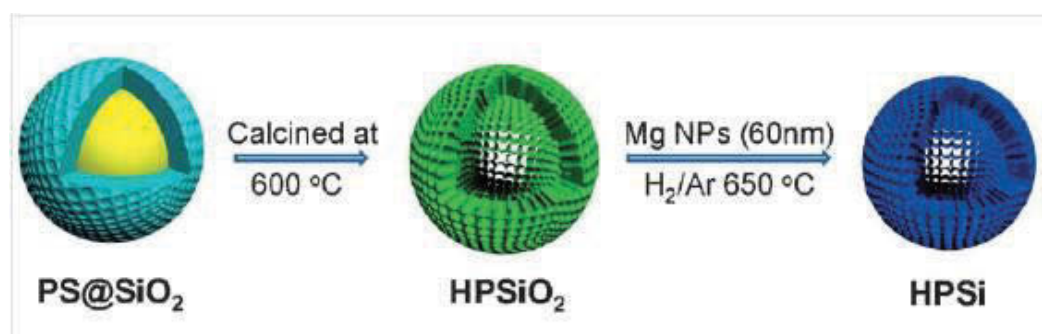
Figure 2.17 Schematic of the preparation of hollow porous Si [179]
