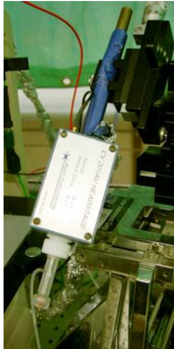
Figure 2.14: View of electrode and headstage. The recording electrode (lower left corner) connected to the headstage input mounted on a micromanipulator (top right corner). A thin polyethylene tube used for suction is attached to the microelectrode holder (bottom left).
