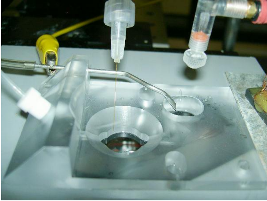
Figure 2.13: Patch-clamp perfusion bath. The main compartment of the perfusion chamber was used to hold the coverslip in place and continuously bathe the neurons in external solution, which flowed in to the chamber via an attached tube on the left of the chamber. The fluid overflow passed into a smaller secondary chamber where it was sucked out by a metal tube to a waste reservoir by a suction pump. Cells were perfused via a perfusion needle delivering a controlled volume of solution into the main chamber. Note: The bath electrode, which would sit in the secondary chamber, is not shown in this photo.
