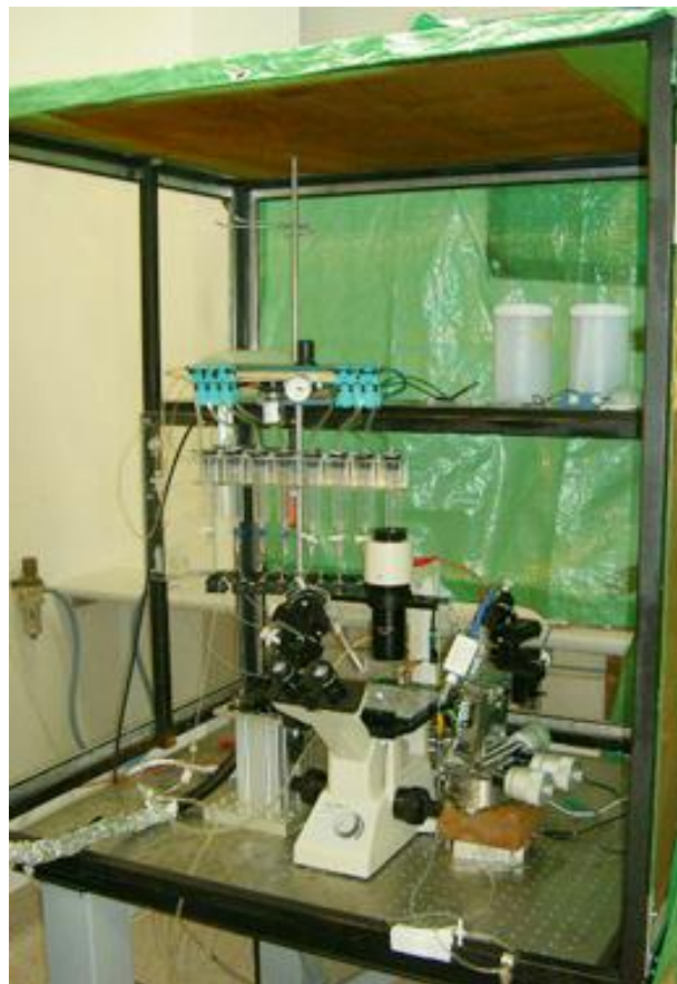
Figure 2.15: Electrophysiology apparatus. The apparatus was placed inside a metal Faraday cage on a vibration isolation table.
