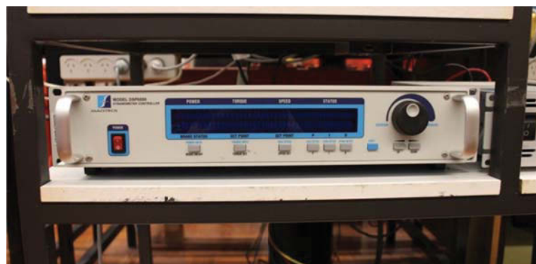
Fig. 3.32 Dynamo-meter controller DSP6000
