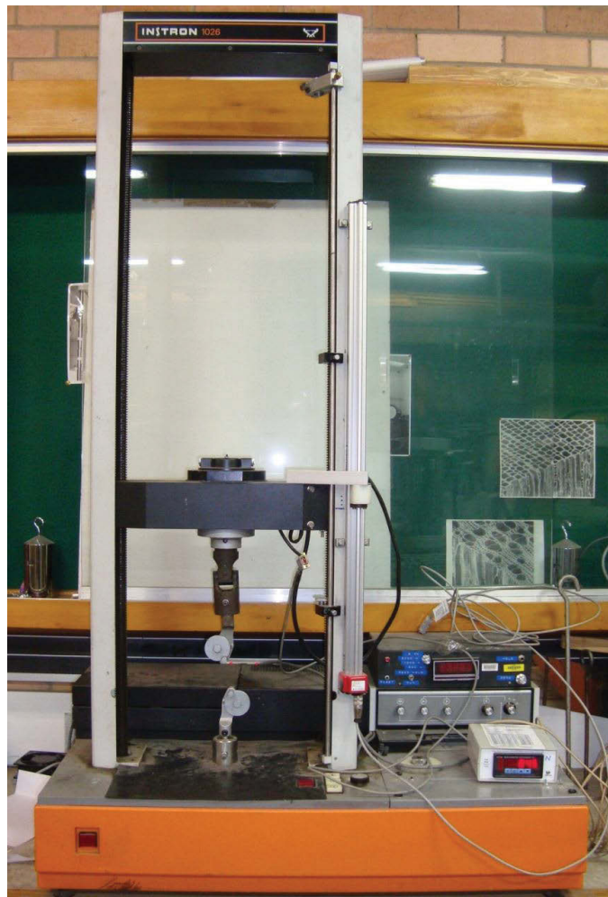
Figure 5.18 Tensile test on wires used as vertical reinforcement
