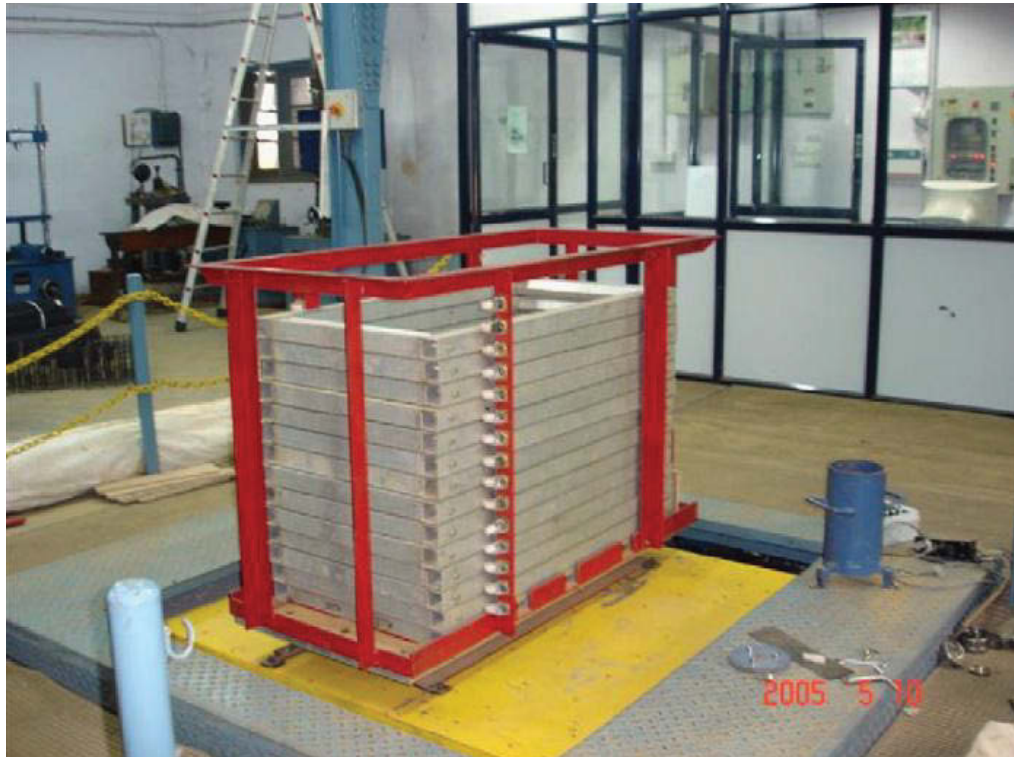
Figure 2.19 Laminar box mounted on a shake table (Krishna & Latha 2007)
