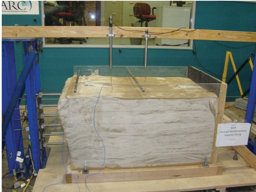
Figure 6.15 Impact of shaking: Model 4 topping failure and its deformed top surface
