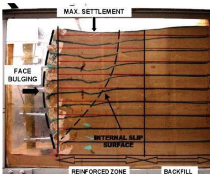
Figure 2.39 Details of the bulging mode and the failure mechanism (Sabermahani, Ghalandarzadeh & Fakher 2009)
