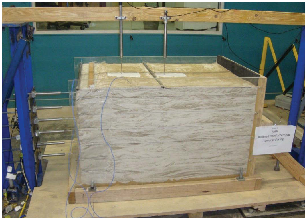
Figure 6.14 Prior to the test: Model 4 and its instrumentation
