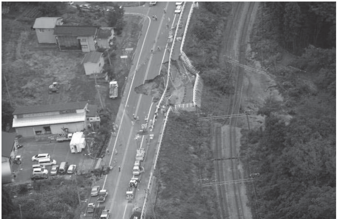
Figure 2.5 Failure of highway and adjacent railway embankment resulting from 2004 Chuetsu earthquake (JSCE 2006)
