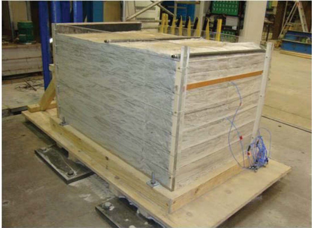
Figure 5.26 Wall with temporary support in facing
