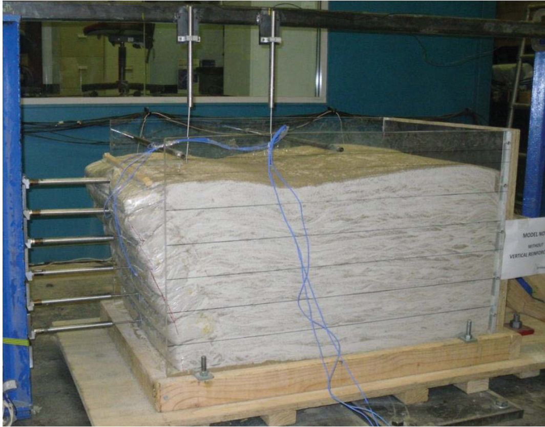
Figure 6.5 Impact of shaking: Model 1 topping failure and its undulated surface
