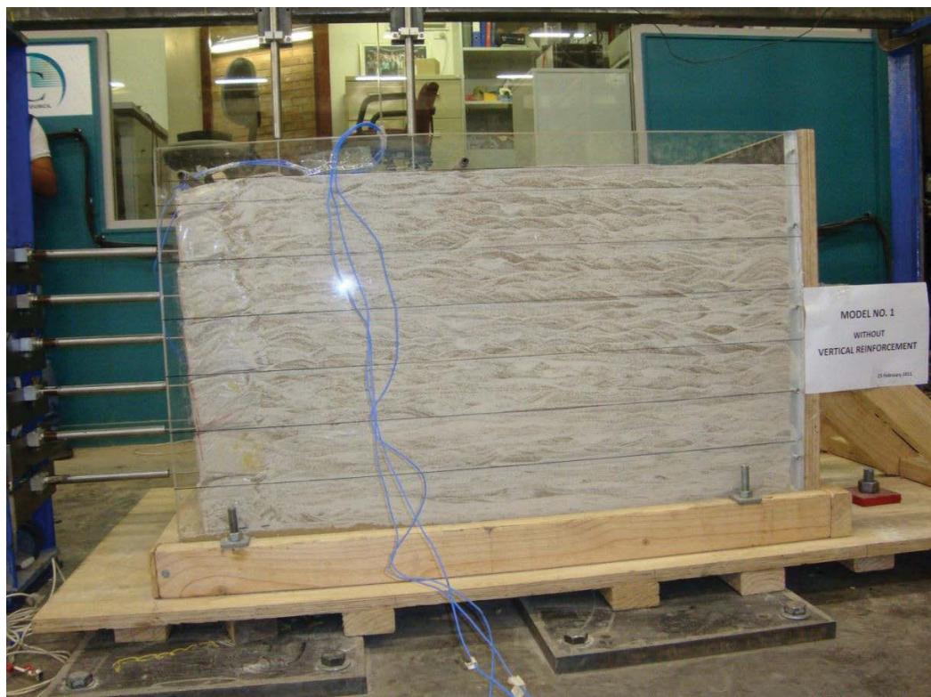
Figure 6.4 Prior to the test: Model 1 and its instrumentation
