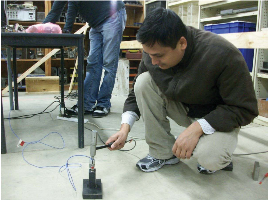
Figure 5.21 Free vibration test to measure the damping ratio
