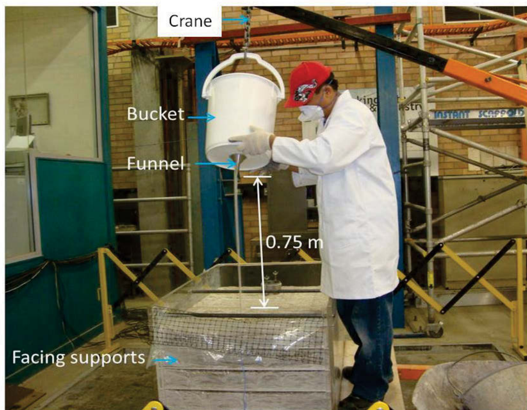
Figure 5.24 Sand backfilling in the model
