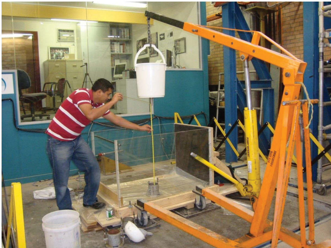
Figure 5.23 Determination of falling height for sand backfilling
