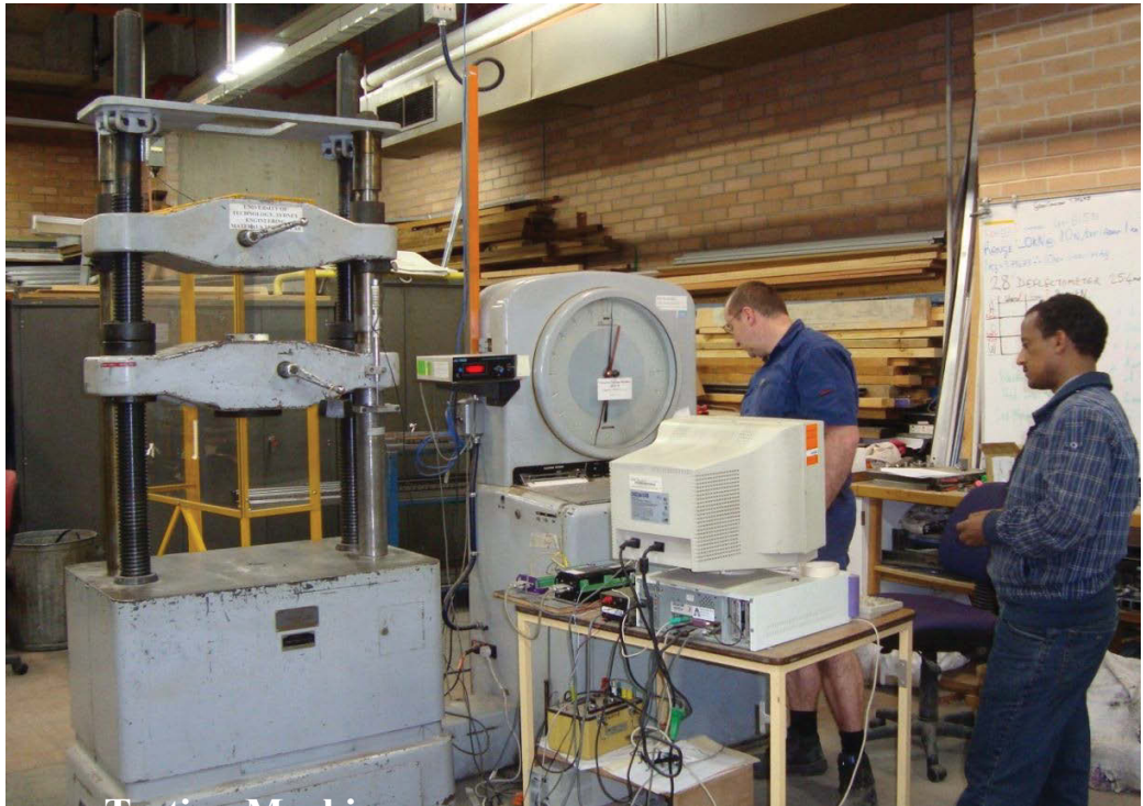
Figure 5.14 The Universal Testing Machine and the associated data acquisition system used for conducting tensile tests
