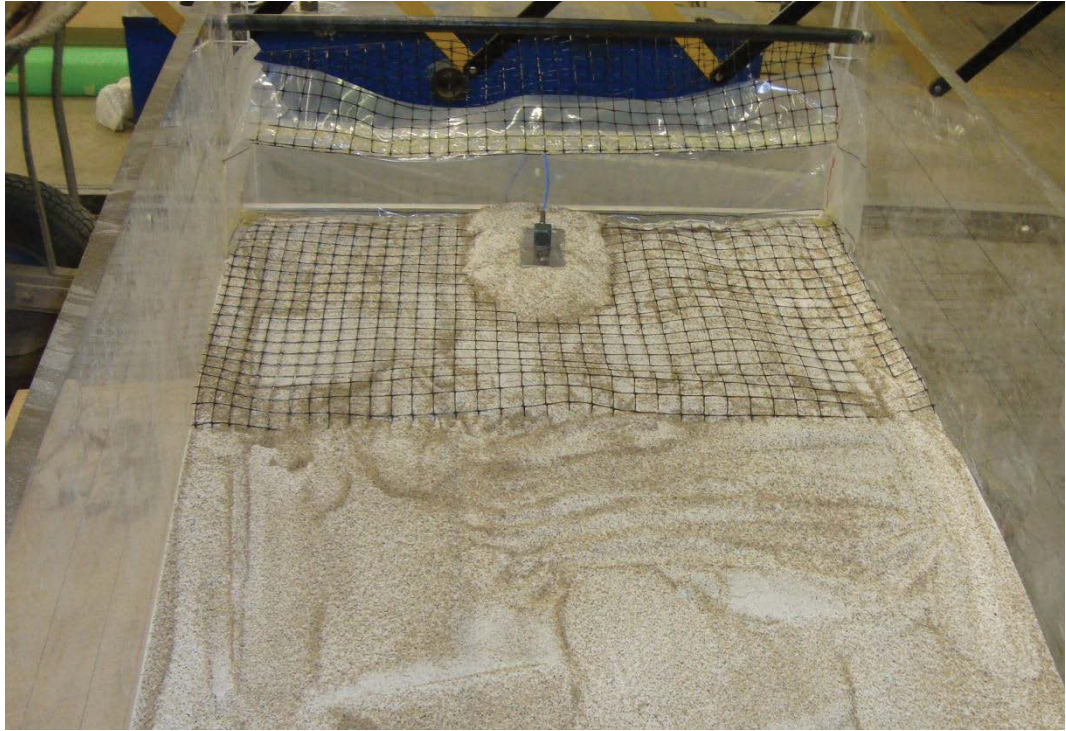
Figure 5.27 Installation of the accelerometer
