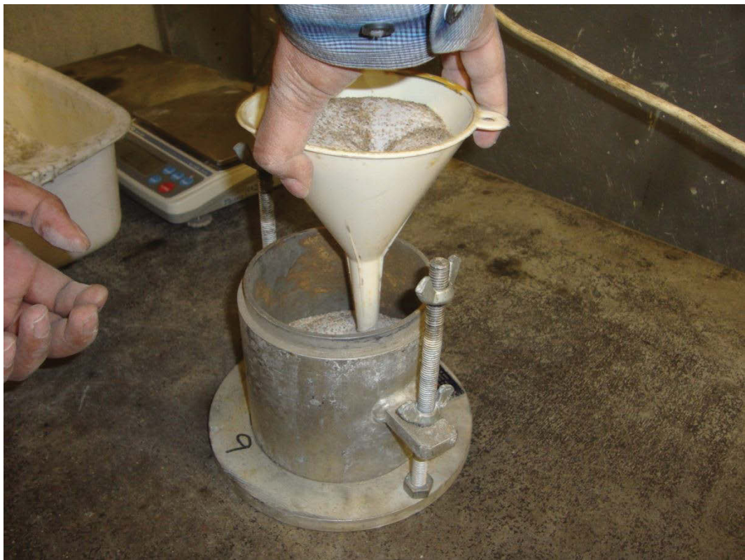
Figure 5.10 Sand placing by pouring funnel to find out minimum dry density
