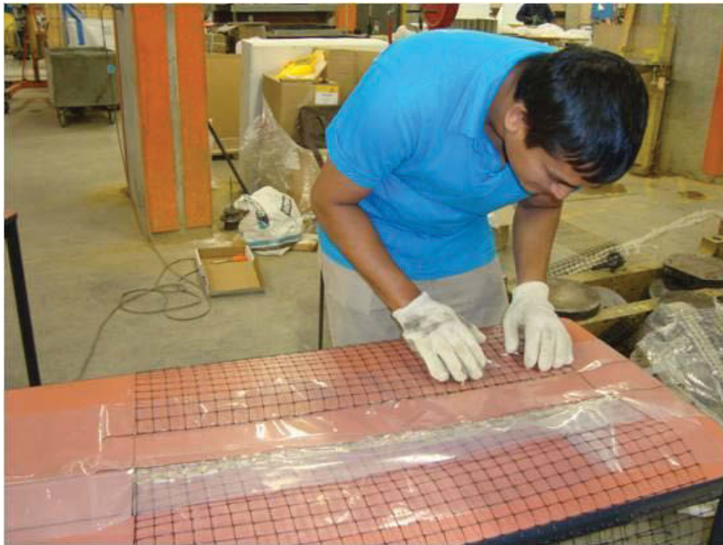
Figure 5.6 Fabrication of facing with reinforcement
