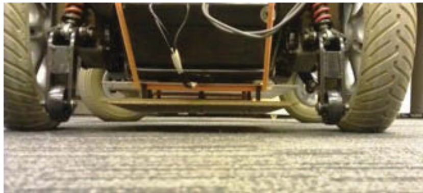
Figure 4-3: Triangular loop bridge reader antenna installed at the base of moving vehicle
