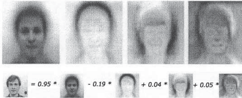
Figure 2.4: Visualisation of the eigenface approach: The first row shows a set of eigenfaces derived from many face samples. The second line shows that a new face can be represented as a linear combination of the eigenfaces. The new feature vector of the test face formed by the coefficients of the linear combination, which is (0.95, -0.19, 0.04, 0.05) . By representing a face image with the coefficients, the dimensionality of face data can be greatly reduced.
