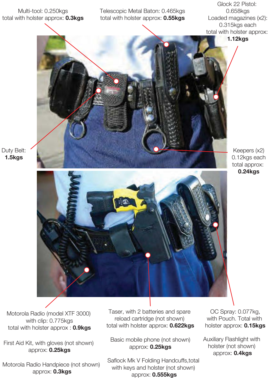
Figure 35. New South Wales General Duty Police officers duty equipment load weights, circa 2010, total weight 12 kilograms
