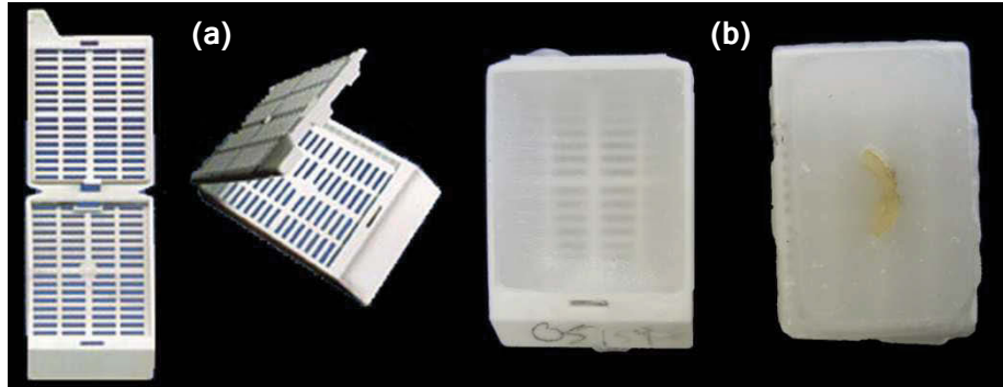
Figure 1-2: (a) Example of a plastic histology tissue cassette; [9] (b) a paraffin-embedded tissue block (front and back).
