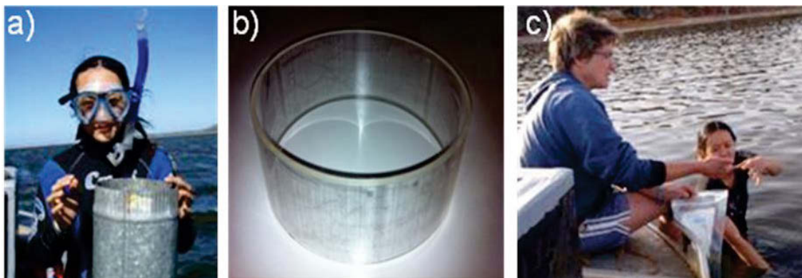
Figure 4.2: Seagrass collection methods showing the two different coring devices: (a) The 20 cm diameter. BROMAR core used to sample in R. megacarpa ; (b) the 14.5 cm diam. perspex core used to sample H. ovalis ; (c) biomass collection process while in the field.
