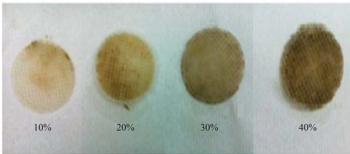
Figure 4.7 Biomass attachment on PE carriers at different filling rates
