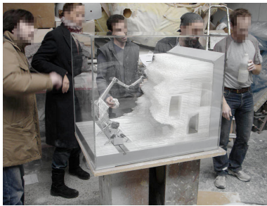
Figure 5: A physical model of the Olzweg project representing a robot placing glass structural elements within an existing courtyard building. (Inaba & Clouette 2006 ,p. 29)
