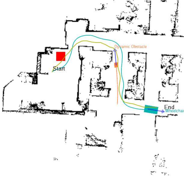
(c) Reacting to the presence of a dynamic obstacle (orange) in the scene.
