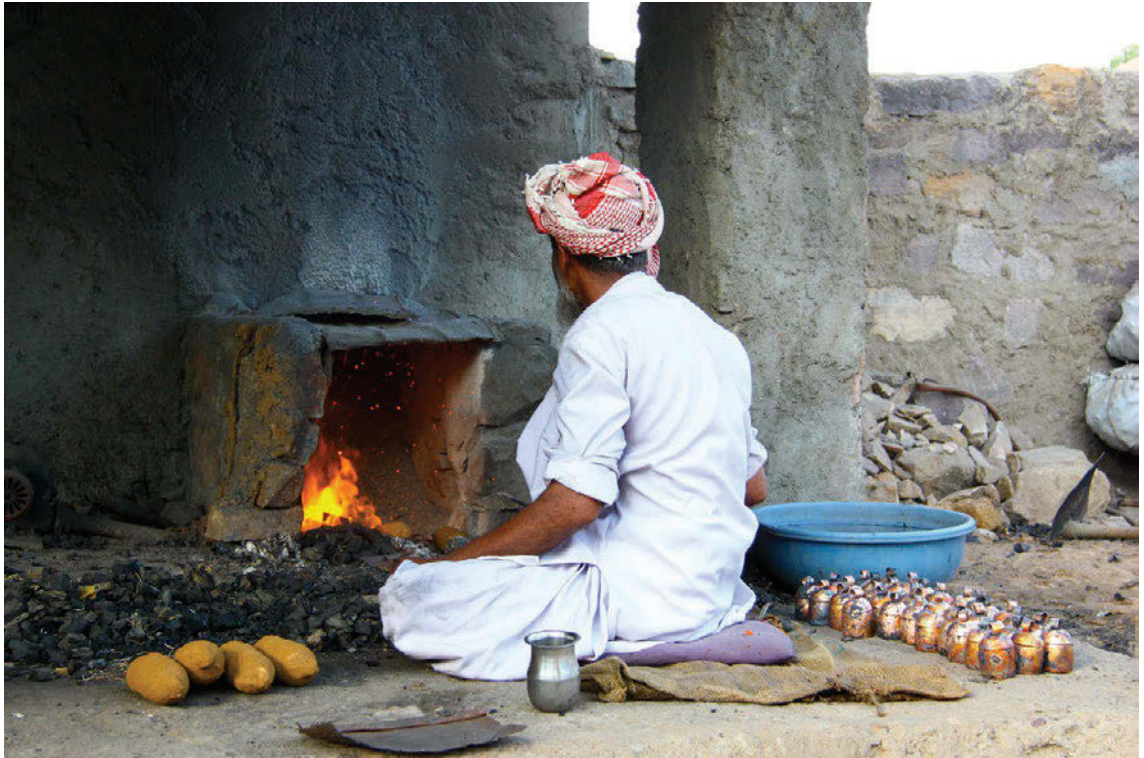
B2.2 Copper bells being fired
