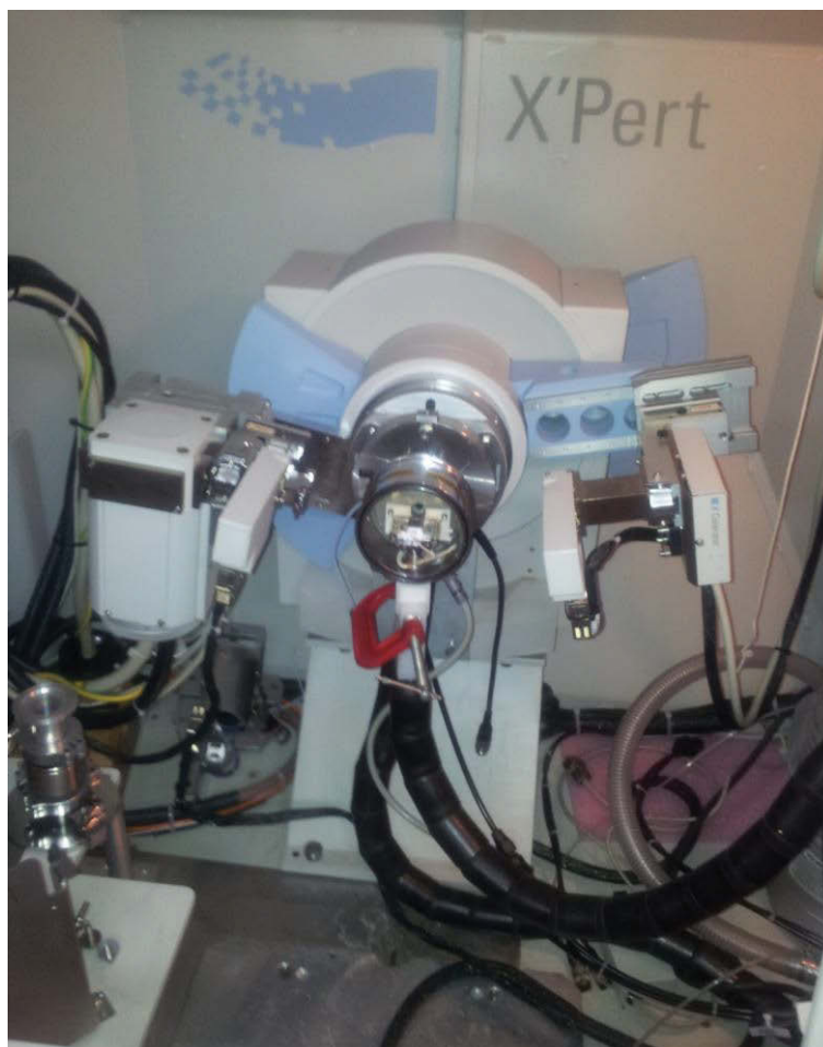
Figure 3.9 Panalytical X'pert Pro X-ray diffractometer was also used with an Anton PAAR TTK 450 temperature stage.
