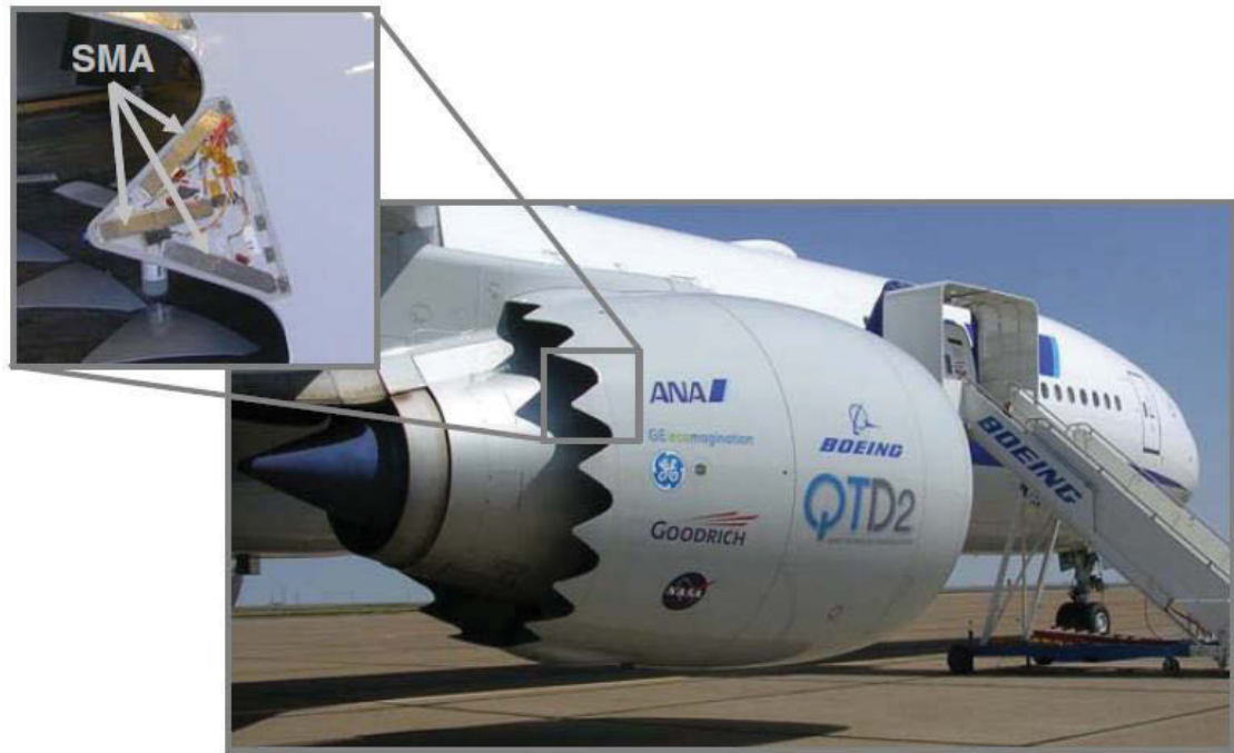
Figure 2.3 SMA actuators used in Boeing variable geometry chevrons [39].
