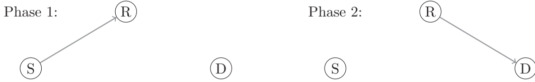
Figure 1.1: The traditional source-coordinated relay model finds an alternate path around a poor link by sending frames via a relay
