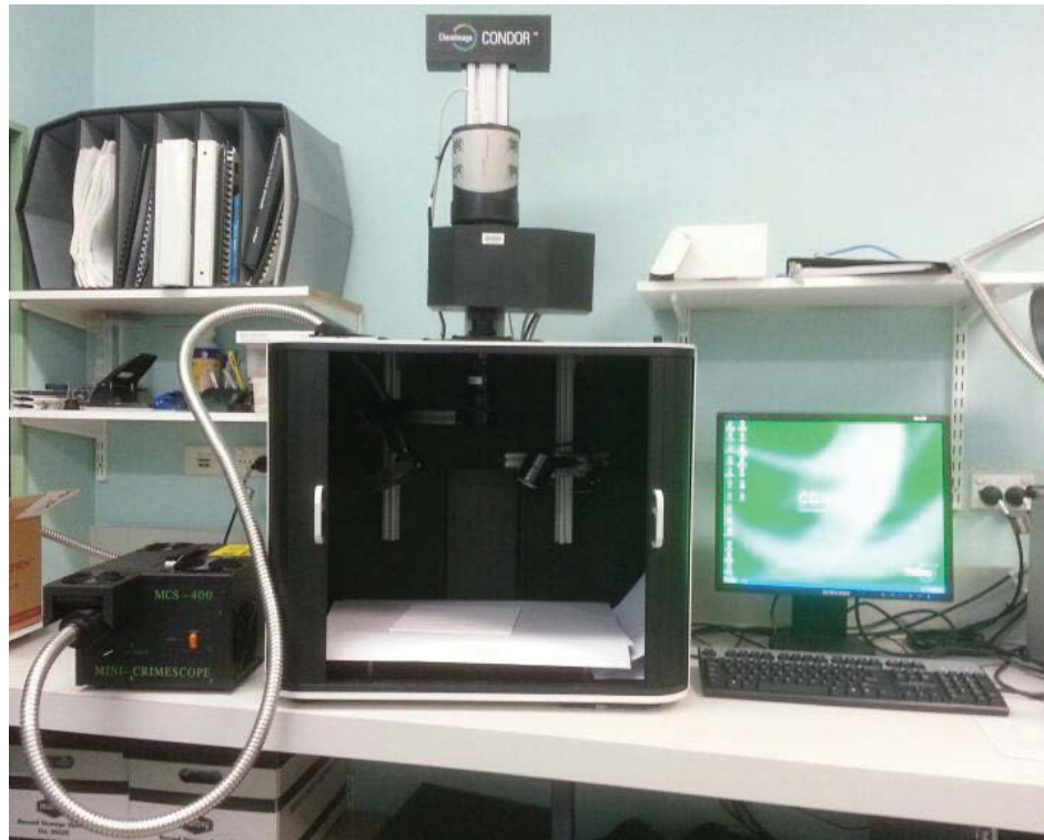
Figure 6-1: The Condor chemical imaging system used in this study.
