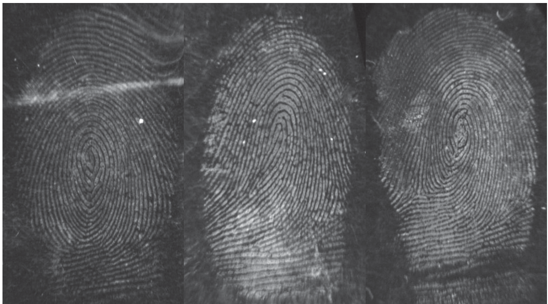
Figure 5-5: PolyCyano UV developed natural fingerprint on polyethylene bags; (left) 70% RH, (centre) 75% RH, (right) 80% RH.
