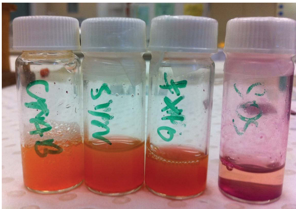
Figure 3-4: STaR 11 suspensions - (l-r) CTAB, synperonic N, triton X-100 and SDS).
