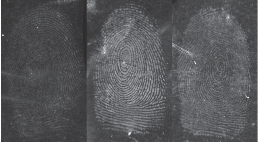
Figure 5-6: PolyCyano UV developed natural fingerprint on polyethylene bag; (left) 15 minutes, (centre) 25 minutes, (right) 35 minutes.
