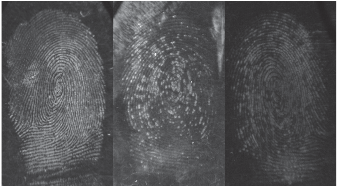
Figure 5-4: Natural fingerprint on polyethylene bags developed with; (left) 0.5 g, (centre) 0.6 g, (right) 0.7 g PolyCyano UV.
