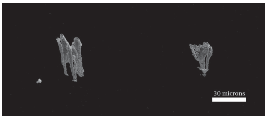
Figure 6.5. Dendritic Pt structures formed via LID of \text{Pt}(\text{PF}_3)_4 . The laser power used to for the left structure was 350 \mu\text{W} , while for the right structure it was 400 \mu\text{W} . It is likely that dissociation occurred in the gas-phase, suggesting a photolytic dissociation mechanism.
