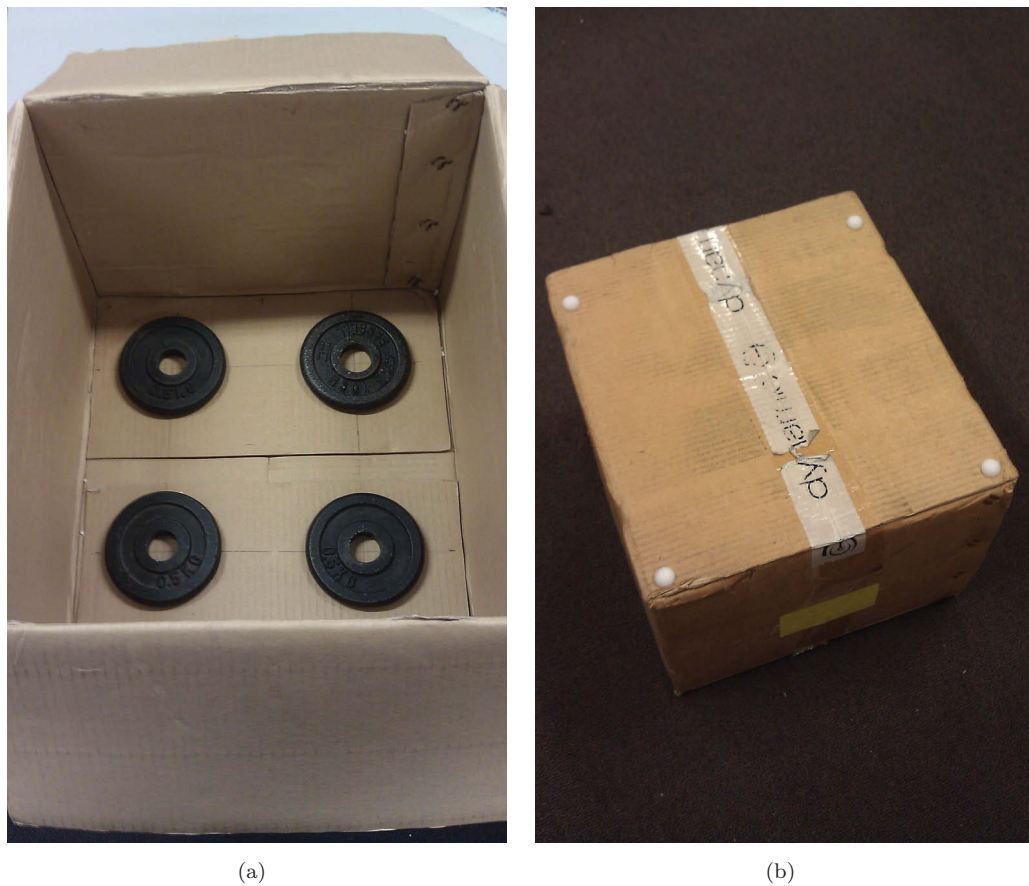
FIGURE 2.30: Sliding object showing (a) an example of mass distribution for balanced support friction and (b) the location of the support points.
