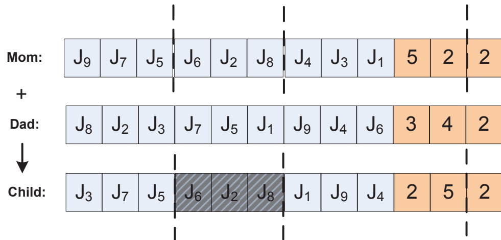
Figure 6-1: Example of using the ORX+A crossover method (Carter and Ragsdale, 2006) for two-part chromosomes
