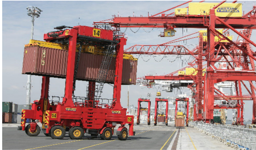
Figure 1-2: ASC transporting a 40-foot container from the quay side as part of a buffer-to-yard task.
