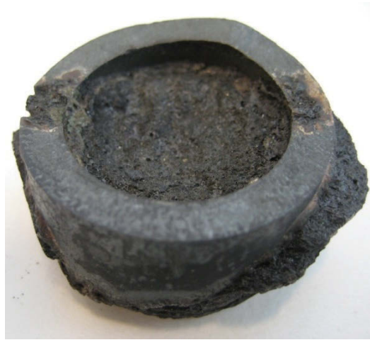
Figure 4.4: Image showing the stainless steel tube with white cast iron bonded to the inner wall of the tube.
