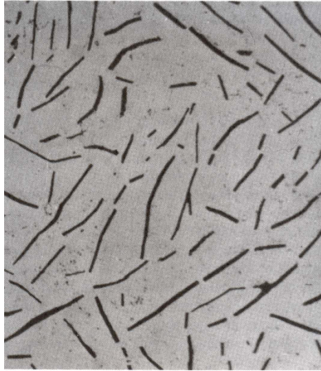
Figure 2.2: Eutectic flake graphite in grey iron (Horizontal Width of Field, HWOF = 200 \mu m)[4].
