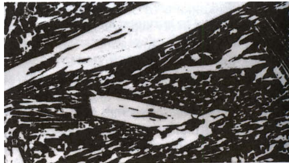
Figure 2.8: Hypereutectic white iron microstructure. Carbides are white and matrix is black (HWOFF = 800 \mu m)[4].
