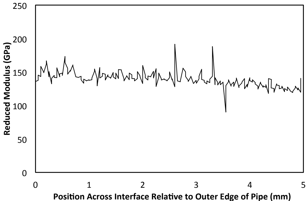
Figure 4.17: Nano-indentation profile showing the reduced modulus of the sample across the interface using a Hysitron Triboindenter 900 nano-indentation system.
