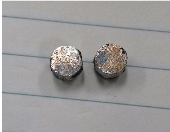
Figure 3.20: Samples coated in Espon HF after 30 mins (left) and 1 hour (right) heat-treatment.
