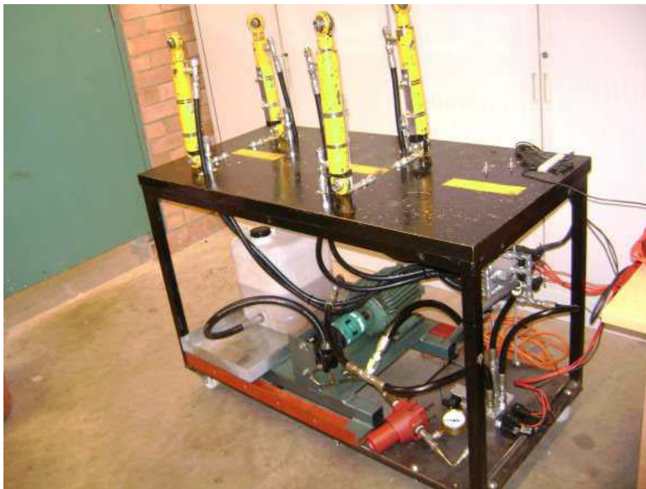
Figure 6.16. Photo of the finished RHIS test rig.
