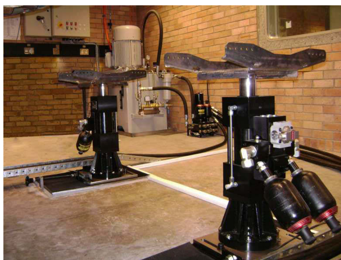
Figure 6.3. Finished cylinders with their motor-pump of the test rig.
