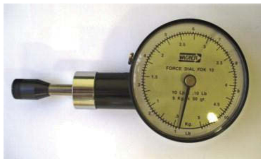
Figure 2.1: An algometer showing the black rubber plunger (surface area of 1 cm 2 ) connected to a spring loaded shaft. The scale indicates the force applied in kilogram (kg) per cm 2 .
