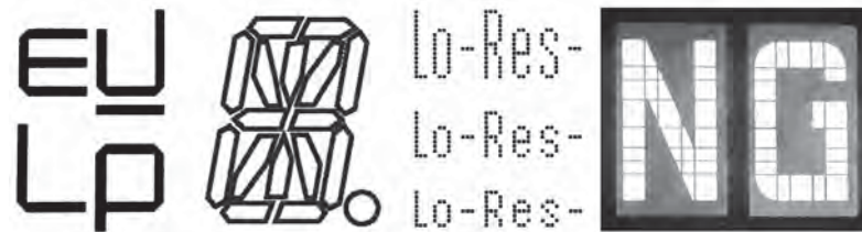
Figure 24 - Monospaced typefaces and gridfonts for different applications (from left to right): Wim Crowel, 1967, the 'New Alphabet'; standard 16-segment LED display schema; Zuzana Licko / Emigre, Lo-Res font, 1985; Masamichi Udagawa / ITP and Sigi Moeslinger / Antenna Design, N.Y.C. subway train identification, over 50 segment LCD.
