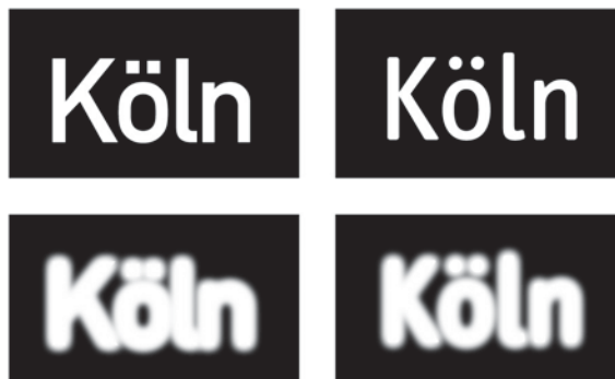
Figure 28 - The effect of radiant light on a backlit sign
