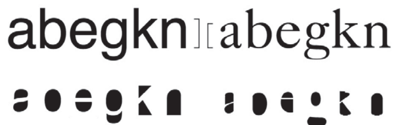
Figure 10 - The x-height as influential factor in rendering clear characters exemplified by the font Helvetica on the left and Centaur on the right
