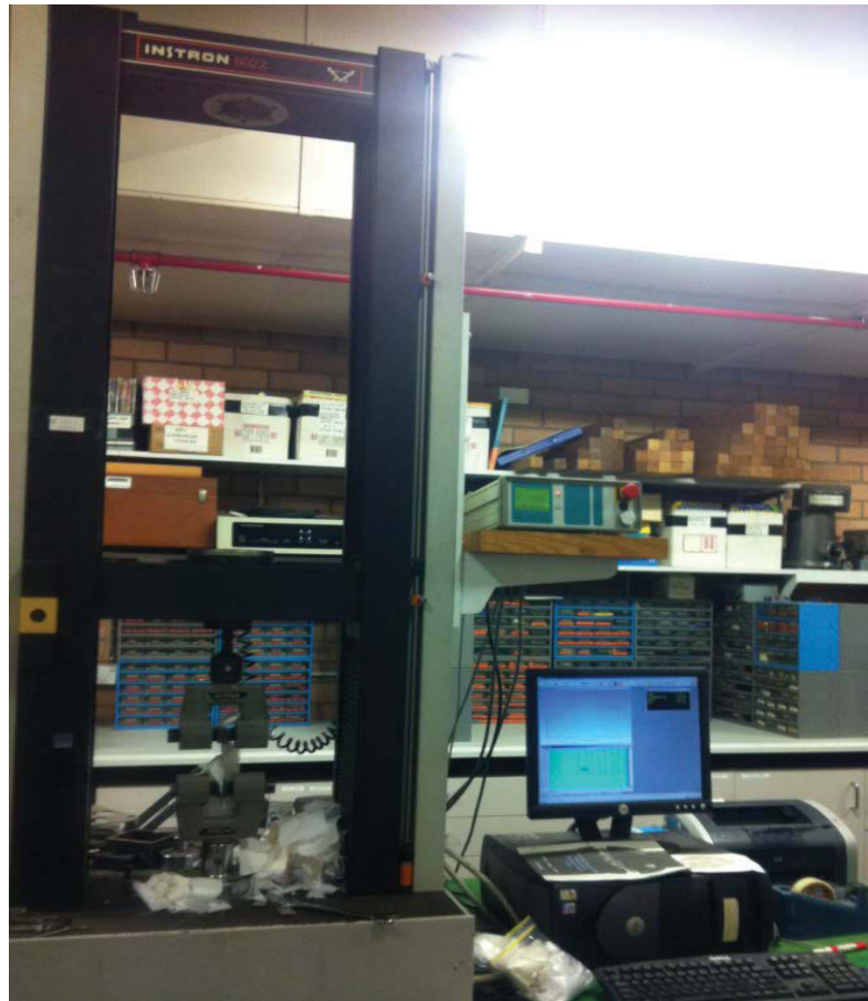
Figure 3.2 Instron 6022 10kN Universal Testing Machine interfaced with computer.
