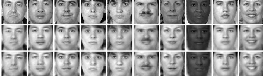
Figure 5.3: low-rank image compression via BRP on FERET: BRP compresses 700 40 \times 40 face images sampled from 100 individuals to a 700 \times 1600 matrix with rank 60. Upper row: Original images. Middle row: images compressed by SVD (6.59s). Bottom row: images compressed by BRP (0.36s).
