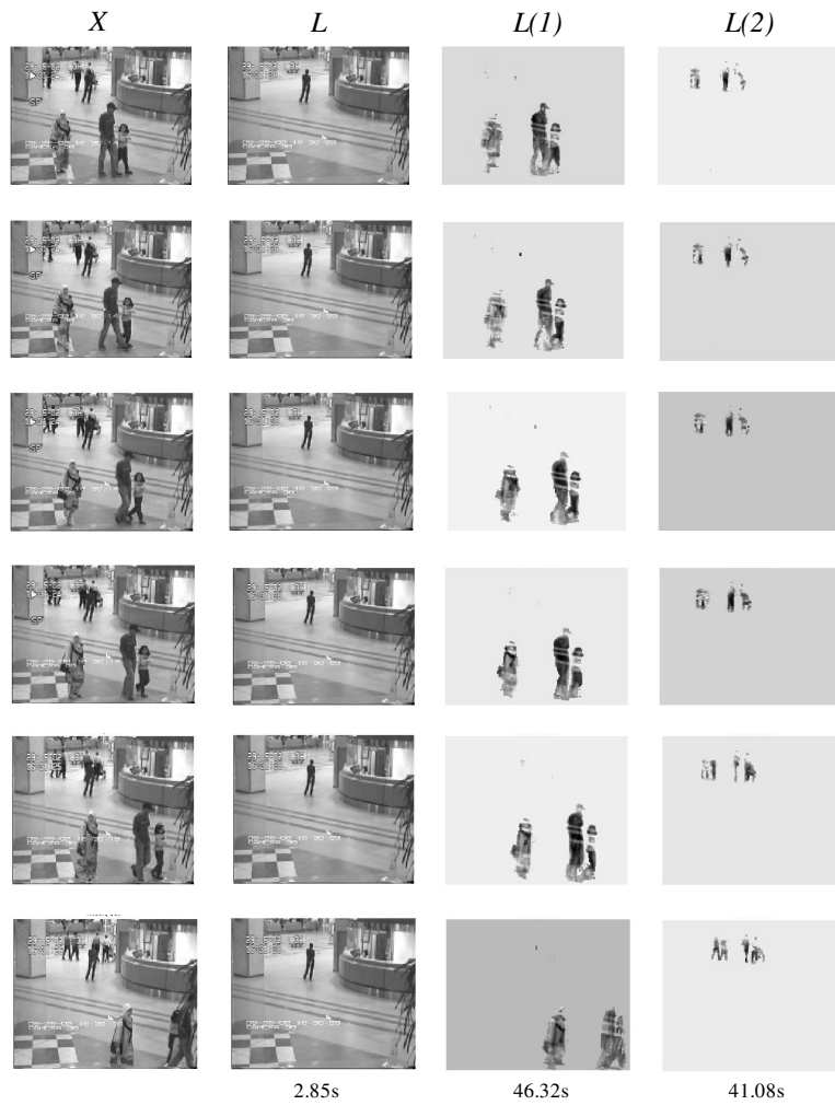
Figure 9.1: Background modeling and object flow tracking results of a 50-frame surveillance video sequence from Hall dataset with resolution 144 \times 176 .
