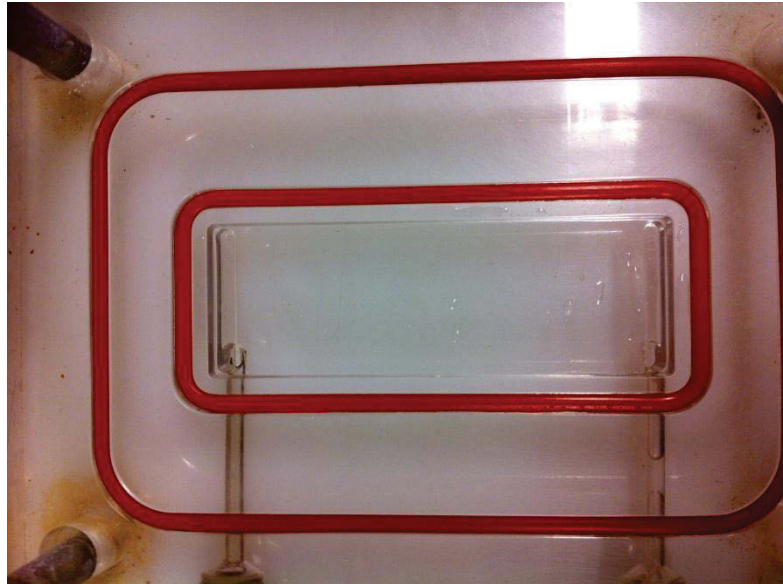
Figure 3.2: a) Close up of FO membrane cell, b) Inside the FO membrane cell
