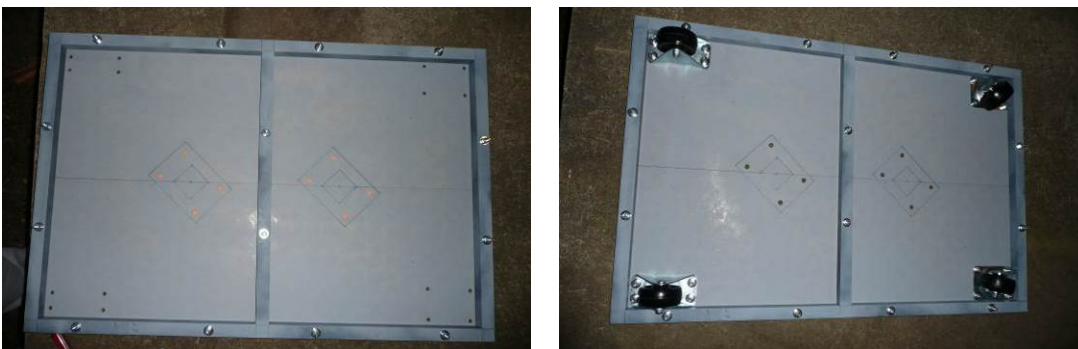
Figure 3.13 Construction of filter column filtration system – Painting of the base
