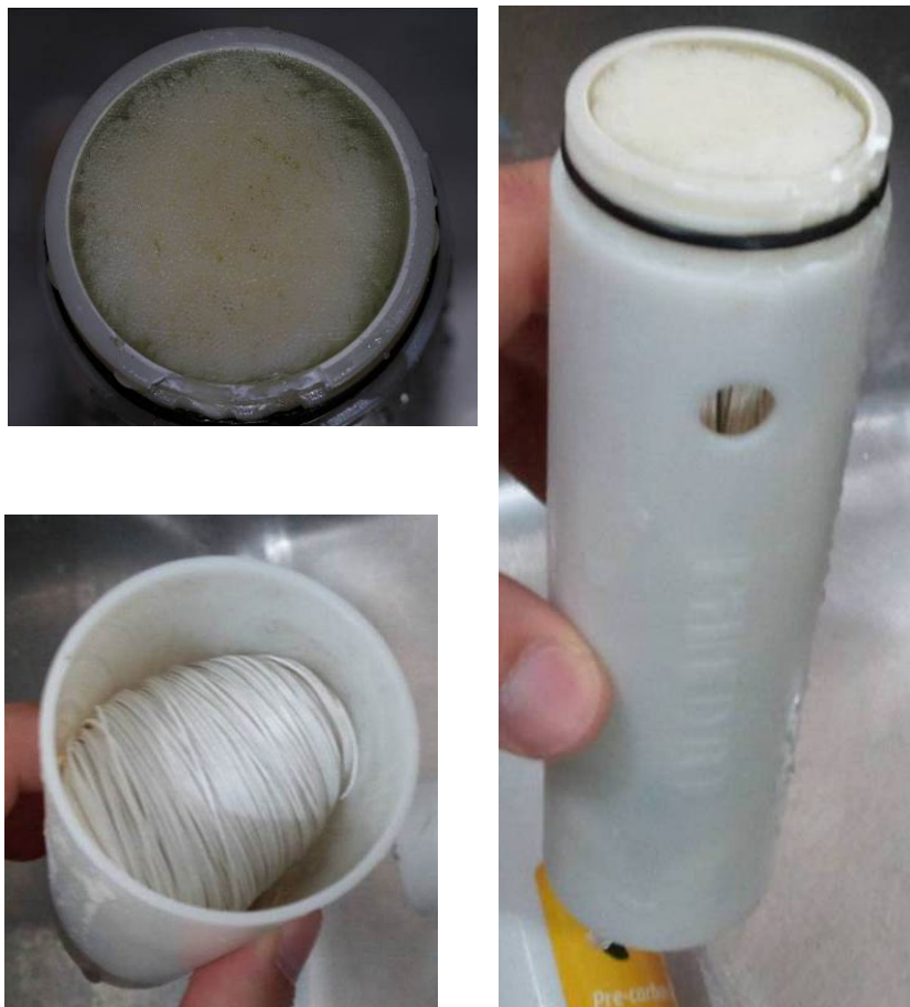
Figure 3.11 Photograph of cartridge filtration system
