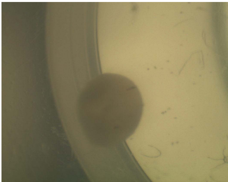
Figure 3-3: A DNA pellet formed after the trial to solubilise using 90% methanol / 10% H 2 O. Image recorded using white transmittance light and viewed at x20.
