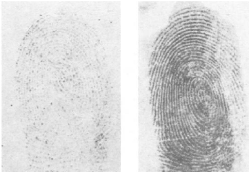
Figure 1-12: MCAR technique as a second step after ninhydrin processing. Ninhydrin development alone (left) and MCAR staining after ninhydrin (right). Taken and reproduced from Ishiyama et al. [122].
