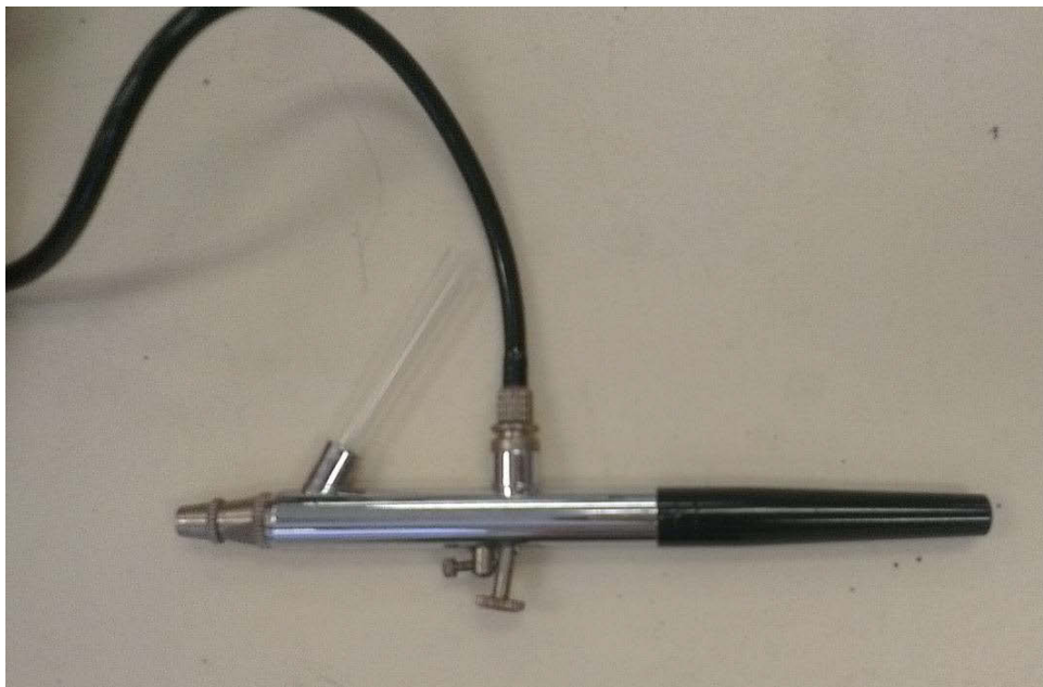
Figure 3-9: Adapted airbrush used to apply aptamer reagent to latent fingerprints on glass slides.
