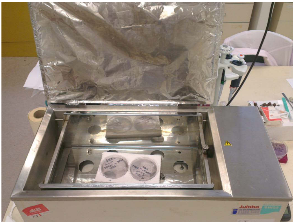
Figure 5-3: Aptamer-based development solutions held at 37 °C using a temperature controlled water bath.
