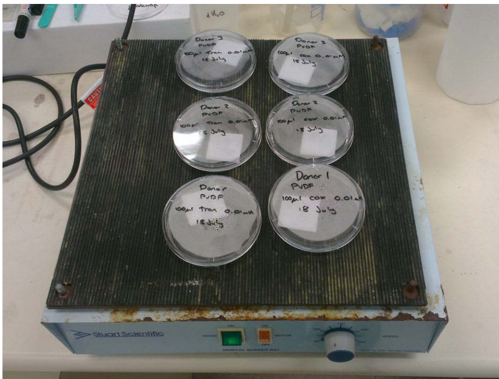
Figure 4-14: Incubation of PVDF samples with aptamer solution (in petri dishes) while being agitated with the use of an orbital shaker.
