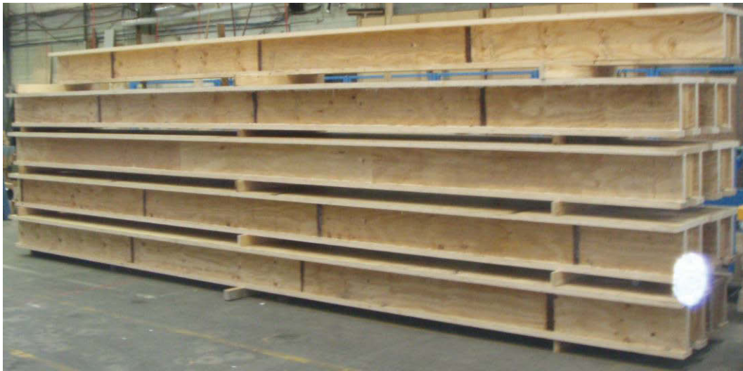
Figure 8.1 Completed prefabricated floor systems
