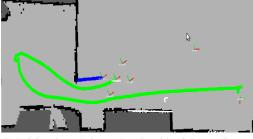
(b) Driving through door sub-task, with minimum distance vector at this instant shown in blue.
