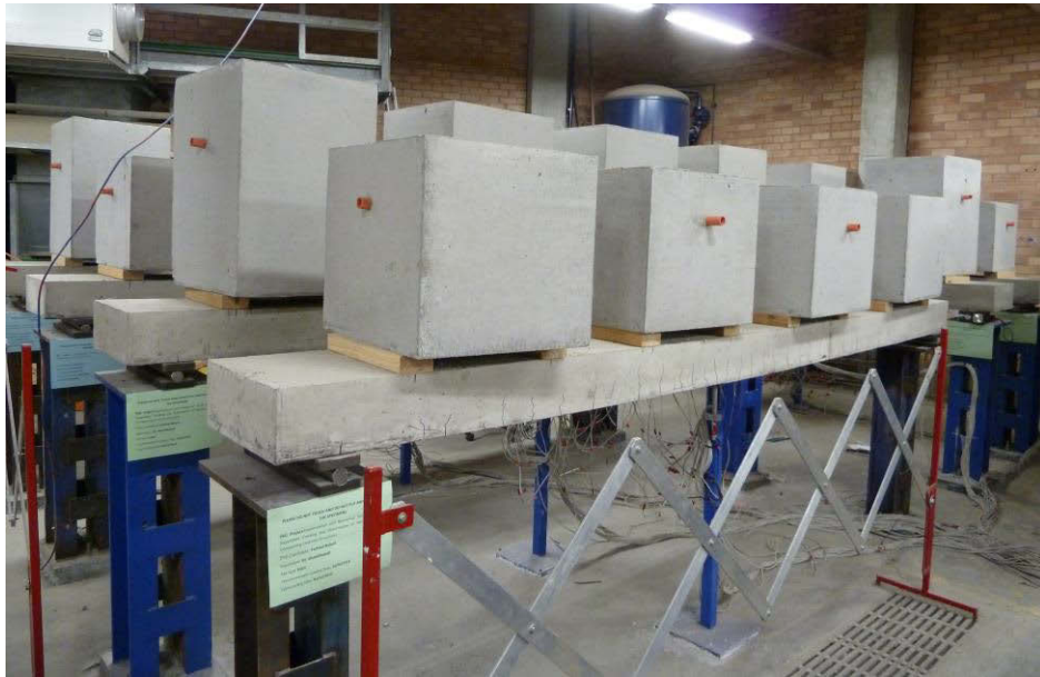
Figure 7.2 Loading slab specimens by concrete blocks
