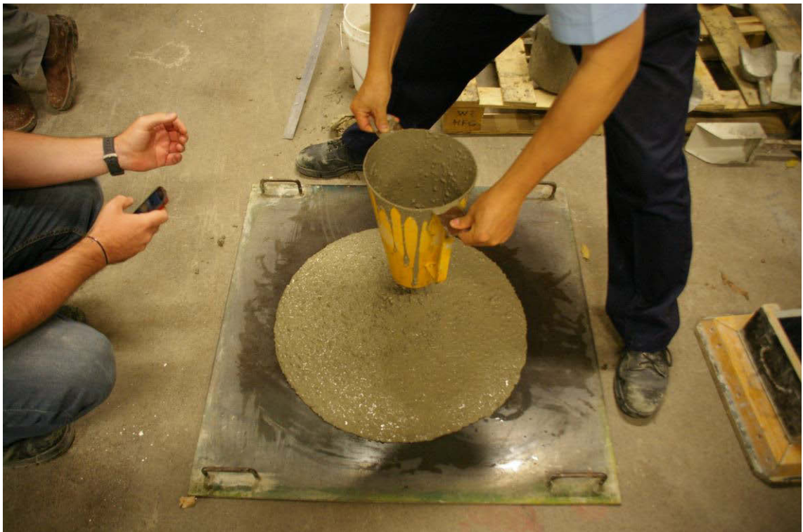
Figure B.1 Slump flow test
