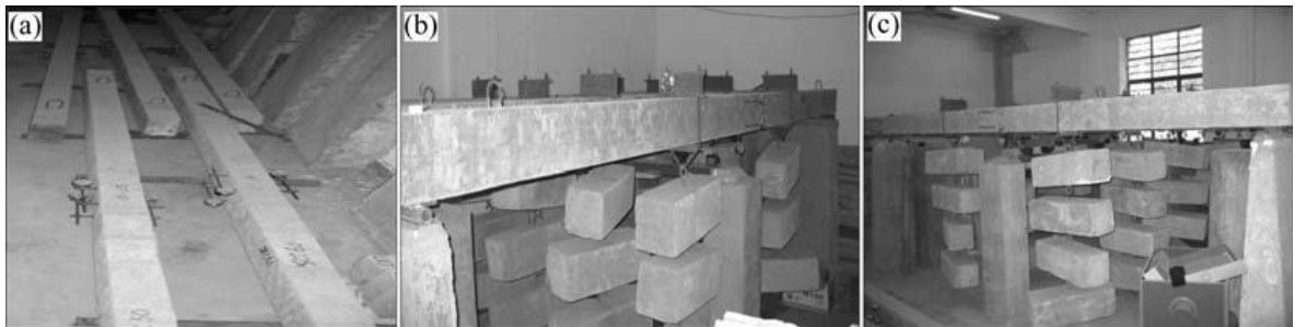
Figure 2.13 Test setup of long term experiment: (a) Shrinkage beam; (b) Simple beam; (c) Continuous beam (Xiao-jie et al., 2008)
