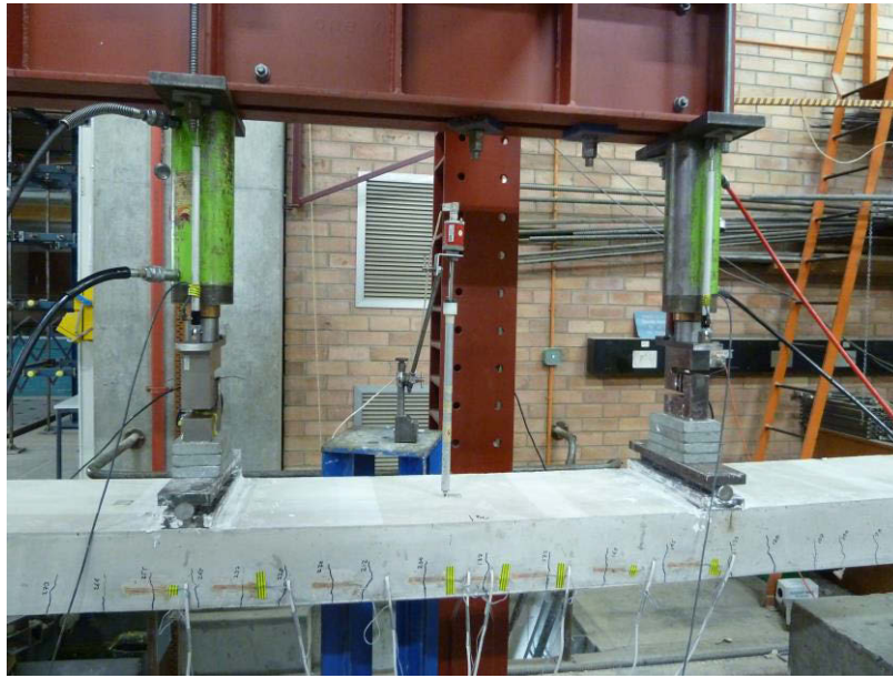
Figure 6.5 General view of loading cells, concrete strain gauges, and LVDT test set-up
