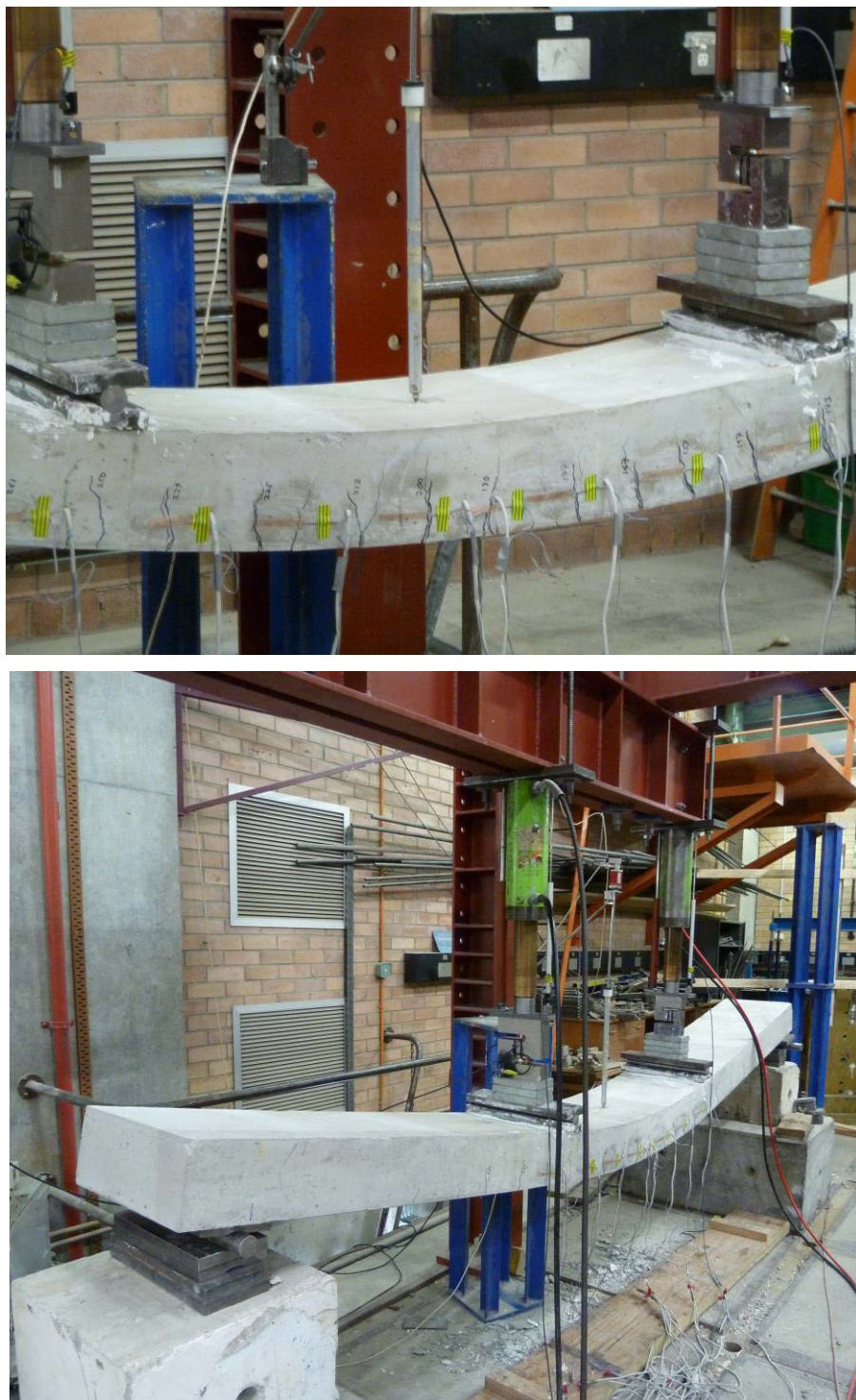
Figure 6.12 General view of slab N-SCC-a failure
