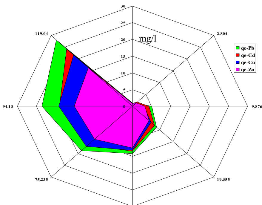
Figure 6.21 Engaged area in terms of capacity of metals in radar diagram for quaternary metals adsorption onto BP.
