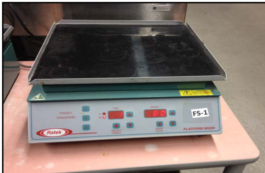
Figure 3.4 A typical platform shaker where all the batch experiments are conducted
