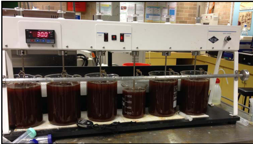
Figure 3.5 A typical flocculator where all kinetics adsorption and desorption experiments conducted
