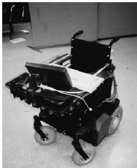
Figure 2.2: Intelligent wheelchair system, University of Michigan (IEEE, 1999)
