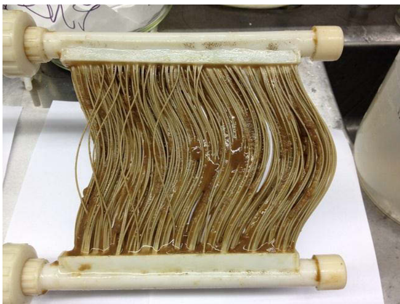
Figure 6.11 The fouled membrane after the MB-SMBR operation (SMBR conditions: aeration rate = 6 L/min; DO = 6.4–7.6 mg/L; filtration rate = 8.83 \text{ L/m}^2 \cdot \text{h} ; HRT = 6h; SRT = \infty ).
