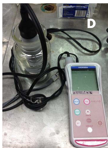
Figure 3.5 The analytical instruments used in this study, including Analytikjena Multi N/C 2000 (A), Hach HQ 40d Portable Meter (B), Photometer NOVA 60 A Spectroquant (C), and Horiba OM-51 Portable Dissolved Oxygen Meter
