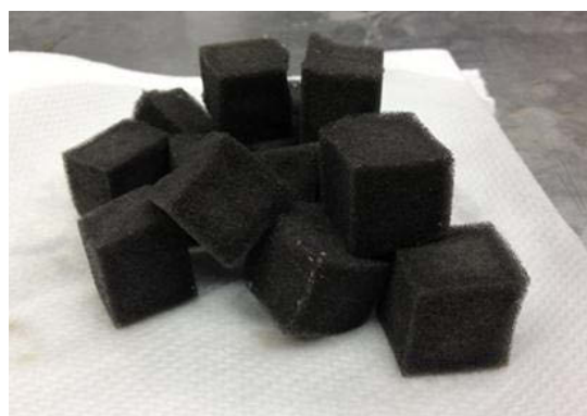
Figure 3.1 The attached-growth carriers (sponge cubes) used in this study
