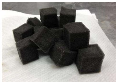
Figure 2.9 Polyurethane sponge cubes with attached-growth biomass
