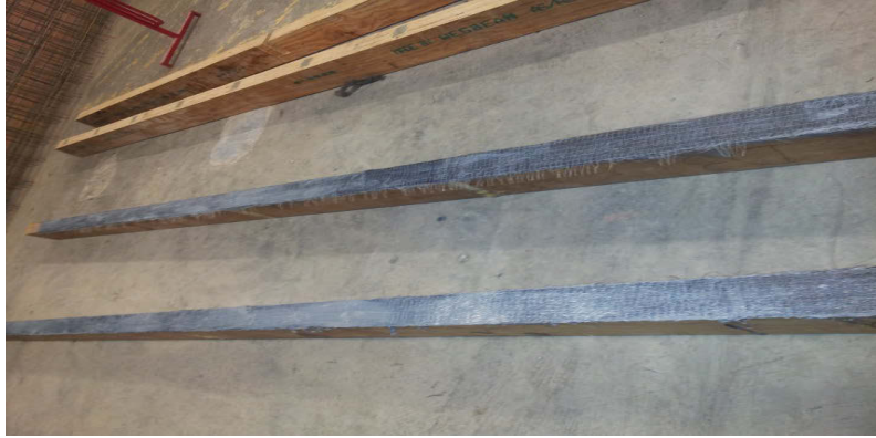
Figure 3.5 LVL Timber beams repaired by CFRP
