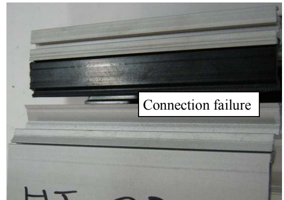
Polyamide pulled away from connection
