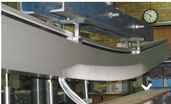
Bending deformation of test specimen
