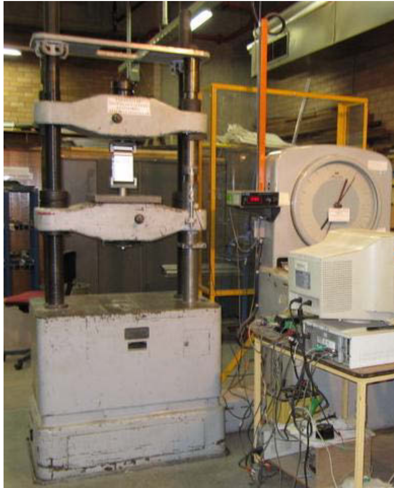
Figure 3.11 Tension test setup full view
