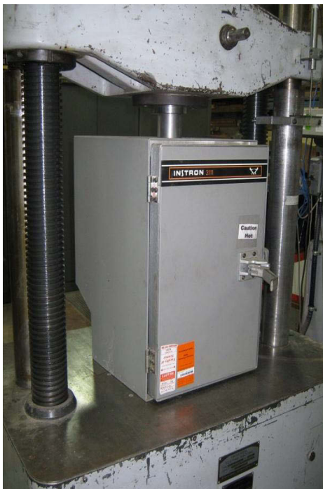
Figure 3.3 Test setup inside temperature chamber
