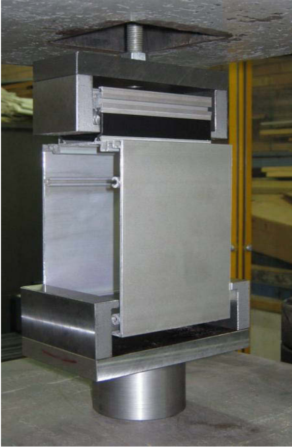
Figure 3.10 Tension test setup sketch and photo at room temperature
