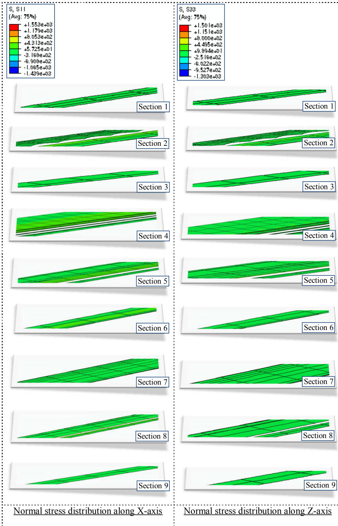
Figure 4.34 Normal stress plot along X and Z axis
