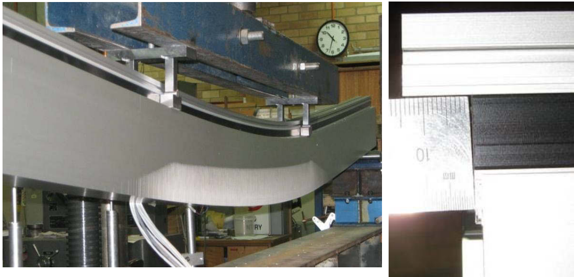
Deformed shape of test specimen
