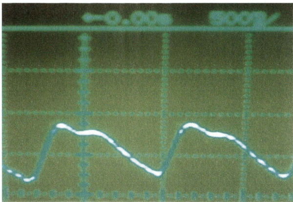
Figure 5.5: PPG signal as sketched by the oscilloscope
