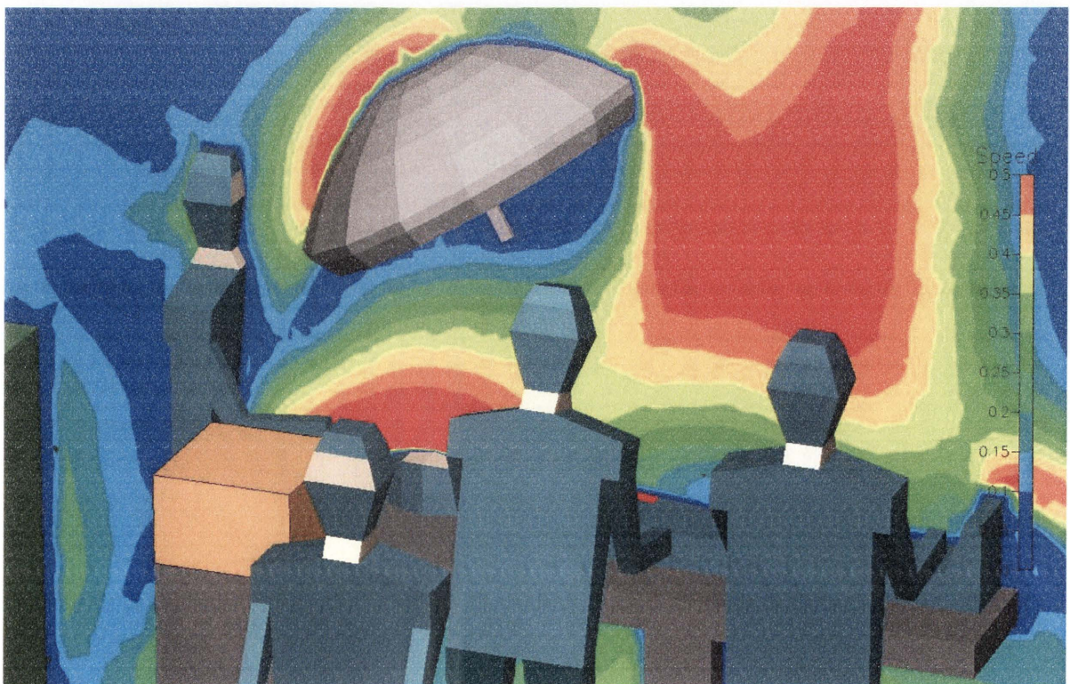
Figure 32. ML1001/C950 Speed (close up) Low speeds induced directly below lamp head, large area of high speed flow induced to the right of the light head, and directly above the light head.
