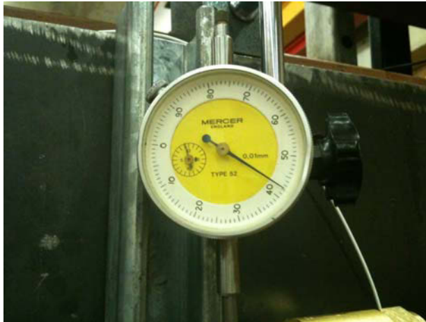
Figure 9.2 Photo of Displacement Meter
