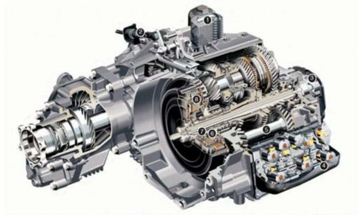
Figure 6-5 Six-speed DCT DQ250[132]: 1) Oil Cooler, 2) Gearshift Mechanism, 3) Oil Pump, 4) Control Unit, 5) Reverse Gear shaft, 6) Input Shaft (G2, G4 and G6), 7) Input Shaft (G1, G3, G5 and Reverse), 8) Wet Dual Clutch
