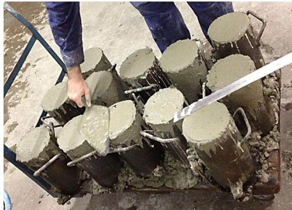
(c) Cylinders required for compressive test
