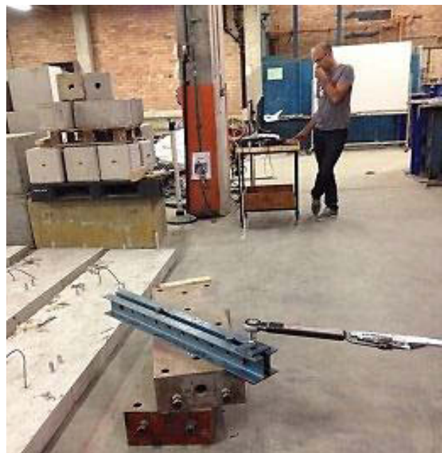
(d) Connecting the instrument to data acquisition machine & tightening the bolts
