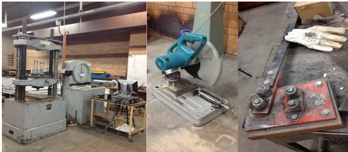
(a) 50-tonne tensile test machine
