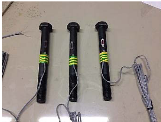
(a) Mounting strain gauges on bolts
