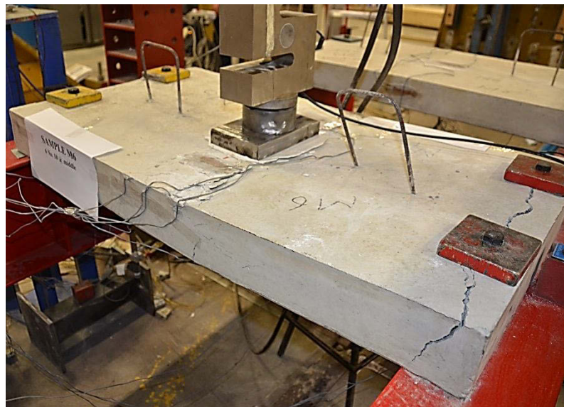
(c) Connection failure accompanied by crushing of concrete
