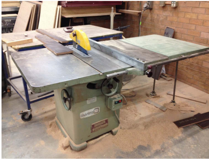
(a) Saw table for cutting the timbers
