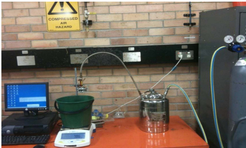
Figure 3.9. UF-MFI experimental set-up photo ( Jeong et al., 2013)
