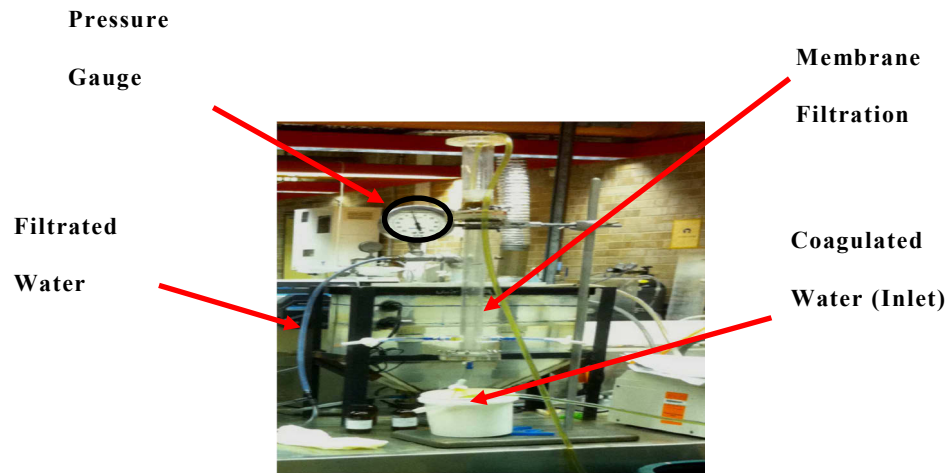
Figure 3.11 Bench scale membrane system
