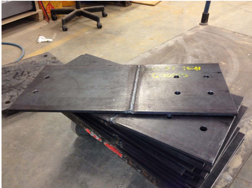
Figure 4-2: Welded joints specimen
