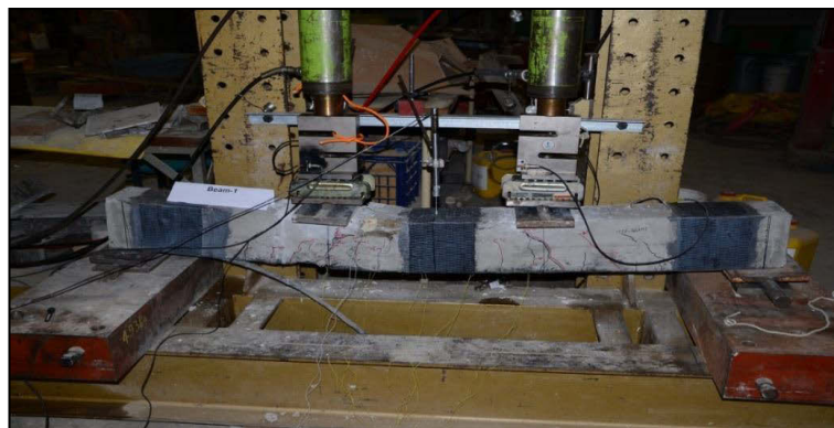
(a) Failed repaired Beam 1
