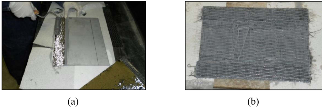
Figure 3.14 (a) FRP application on mould and (b) curing of FRP in lab condition
