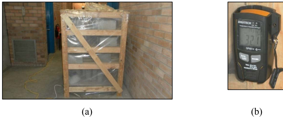
Figure 3.6 (a) Humidity chamber and (b) temperature and humidity data-logger
