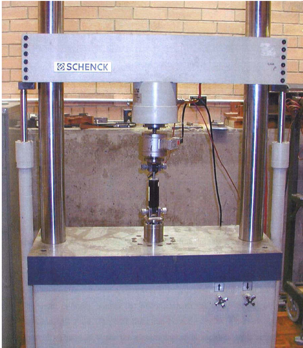
Figure 2.15. MR damper test on Schenck material testing machine
