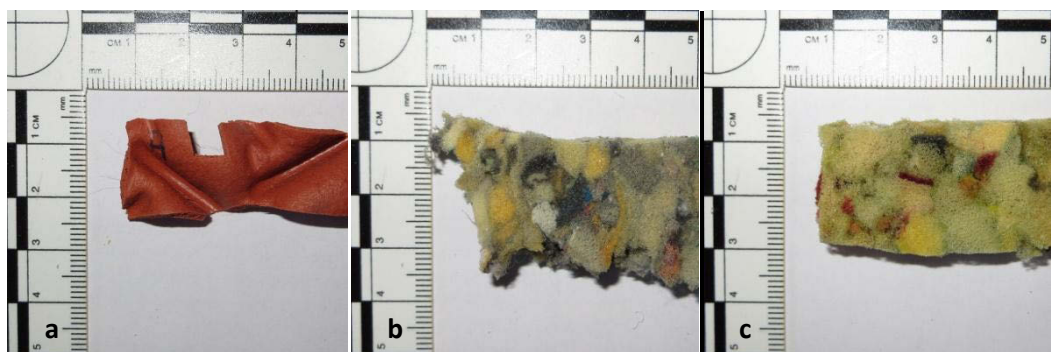
Figure 2.9: Comparison of the foam samples collected from the carpet underlay. a) Room 1, b) Room 2, c) Room 4.
