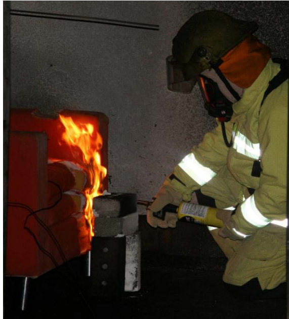
Figure 4.13: An example of the point and mechanism of ignition used throughout the experimental burns.
