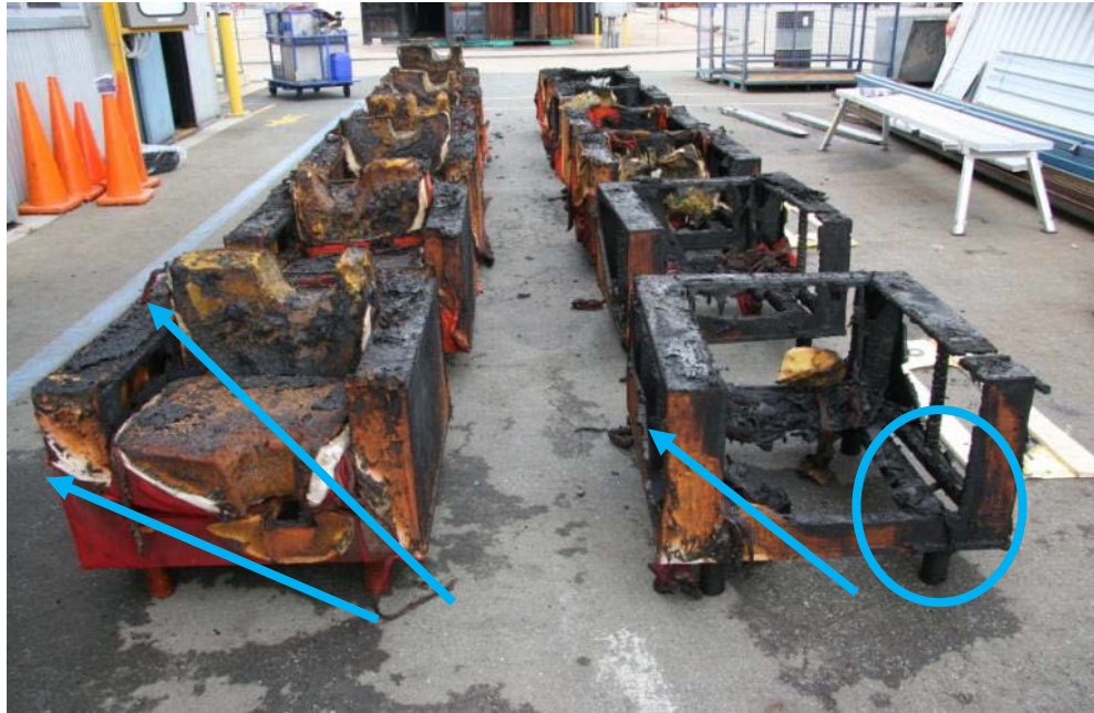
Figure 4.26: Armchairs used in Burns 7–12 post suppression. The circle indicates the area of origin. The narrower arrows indicate a line of demarcation radiating up and out from the area of origin.
