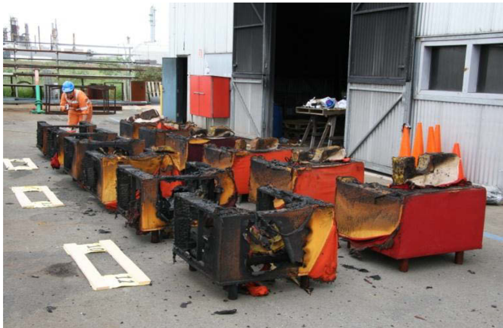
Figure 4.27: Armchairs used in Burns 7–12 post suppression that has been orientated from the area of origin.
