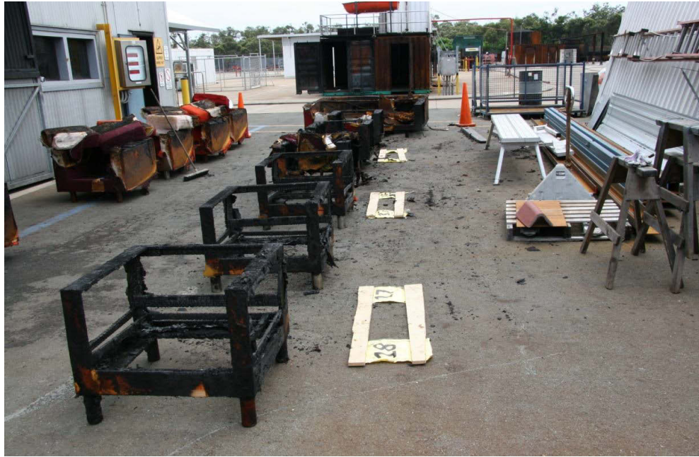
Figure 4.29: Single armchair used for Burns 13 – 18. Burn 18 is in the foreground.
