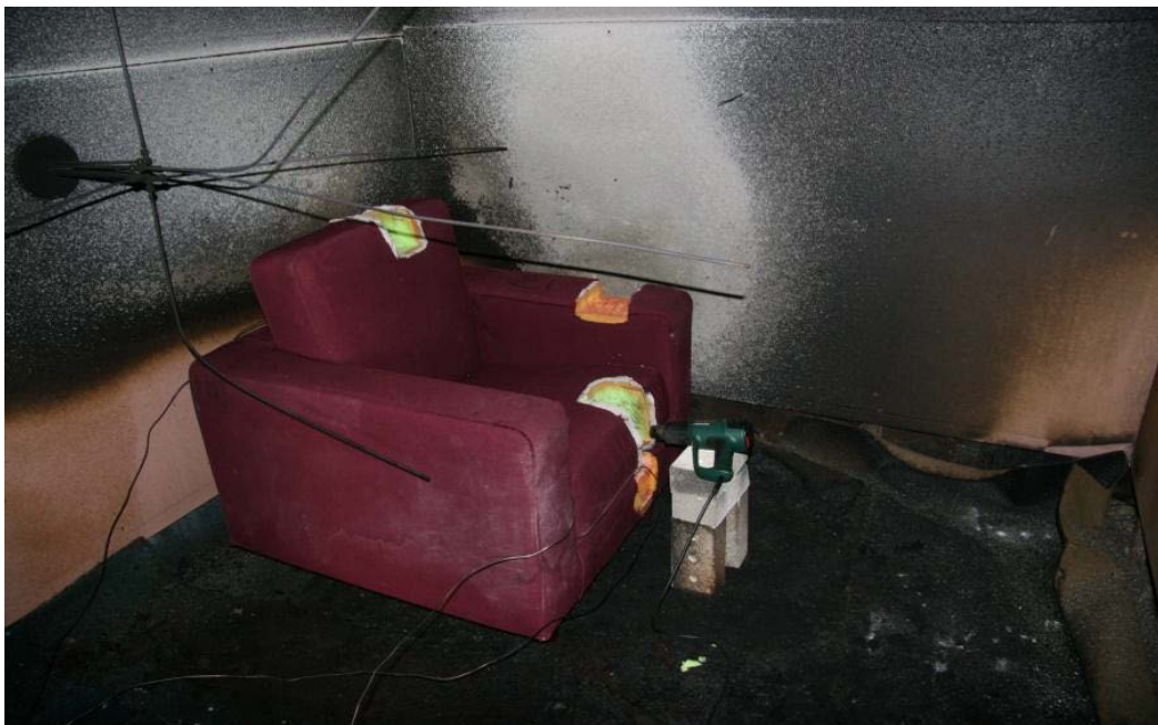
Figure 4.8: Example of how the single armchair, in Burns 13 – 18, was configured.
