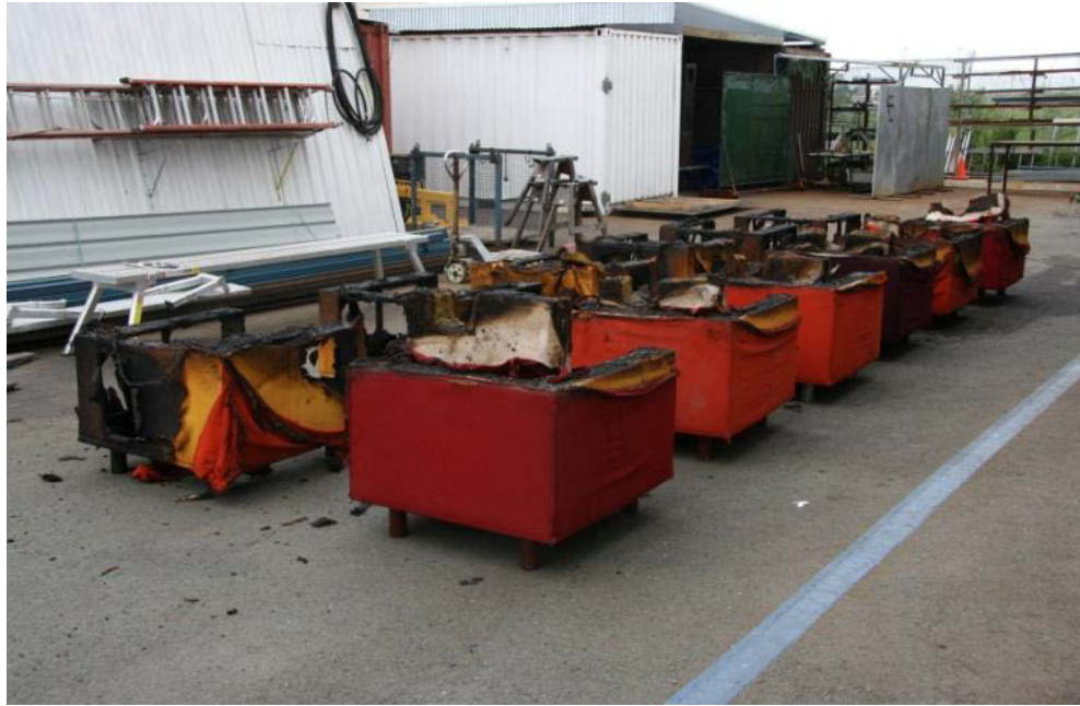
Figure 4.28: Armchairs used in Burns 7–12 post suppression that has been orientated from the end of the armchairs furthest away from the area of origin.
