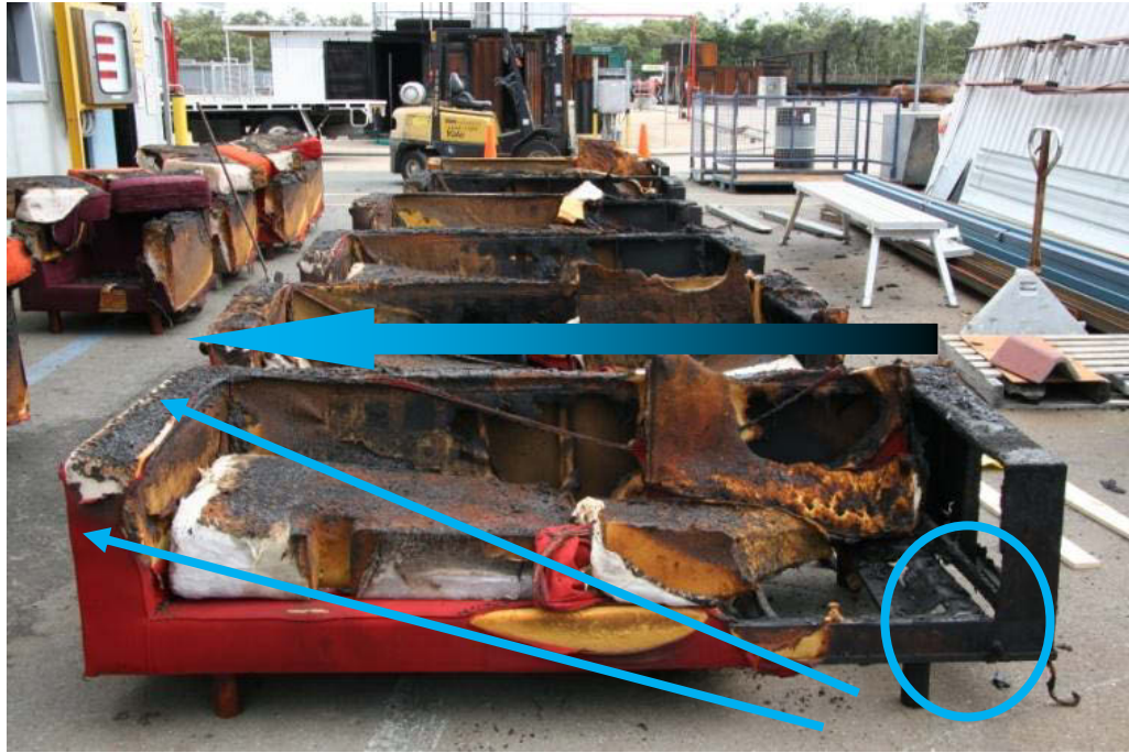
Figure 4.23: Couches used in Burns 1 – 6 post suppression. The circle indicates the area of origin. The narrower arrows indicate a line of demarcation radiating up and out from the area of origin. The larger colour graduated arrow indicates the decline in damage to the couch moving away from the area of origin.
