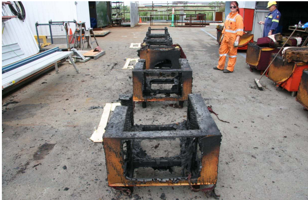
Figure 4.30: Single armchair used for Burns 13 – 18. Burn 13 is in the foreground.
