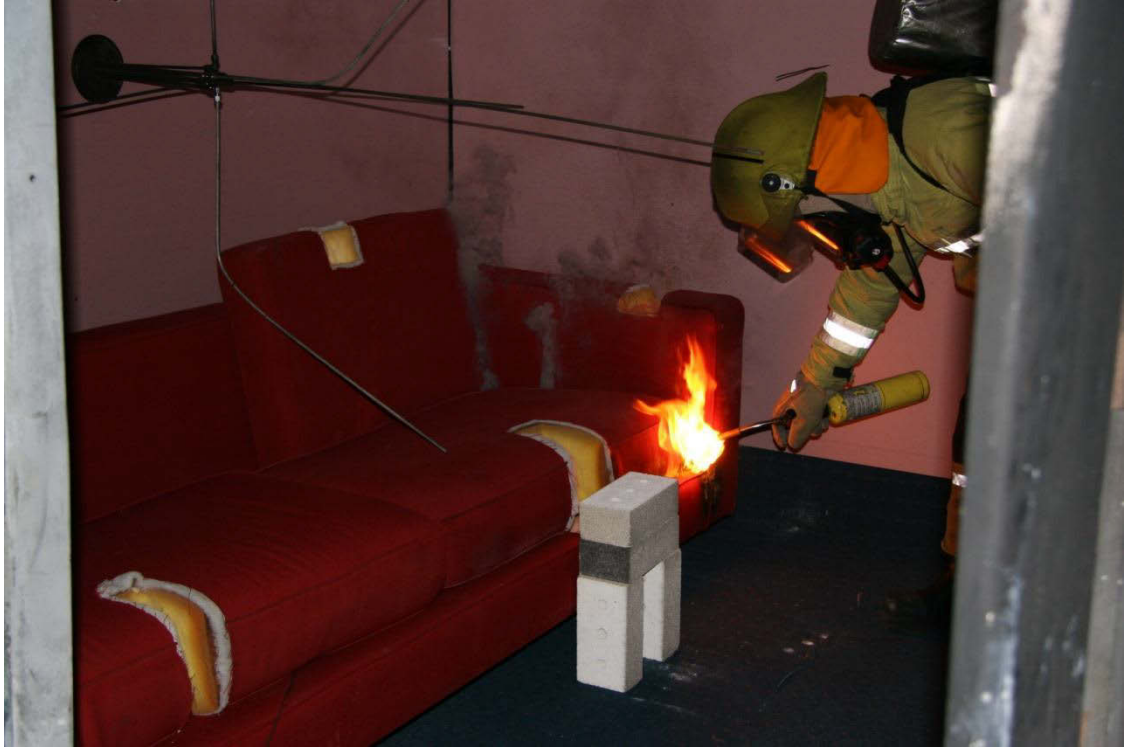
Figure 4.6: Example of three seater couch placement repeated for Burns 1 – 6.
