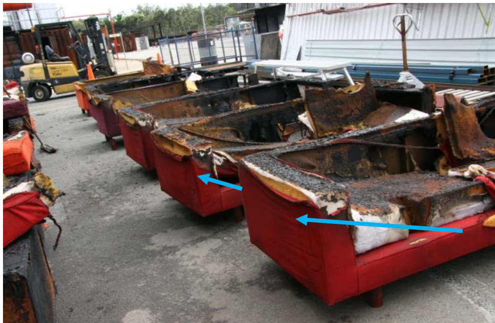
Figure 4.25: Couches used in Burns 1 – 6 post suppression, orientated from the end of the couches opposite the area of origin. The blue arrows indicating the line of demarcation radiating up and out from the area of origin.
