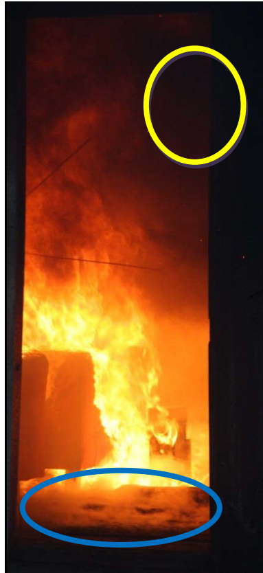
Figure 1.4 The moments immediately prior to flashover.
