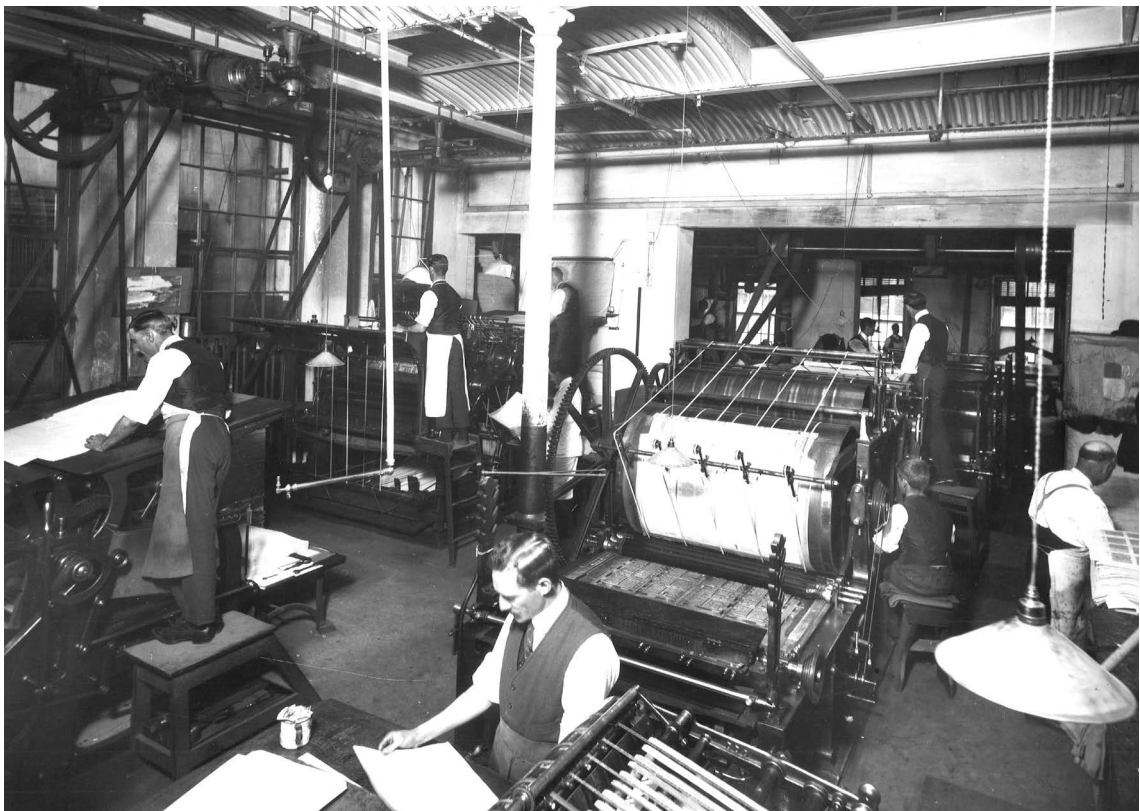
Fig. 5 NSW Government Printing Office pressroom, showing Whitefriars Machine, 1907, Phillip and Bent streets, Sydney. This photograph was reproduced on a large wall in the foyer of the Government Printing Office in 1986, serving as a nod to the Gov's letterpress traditions: a reminder of the types of technology that the Gov had only recently phased out. Courtesy of the Mitchell Library, State Library of New South Wales, Sydney. SLNSW call no. Government Printing Office 1 – 10940. With thanks to Richard Peck for the print.
