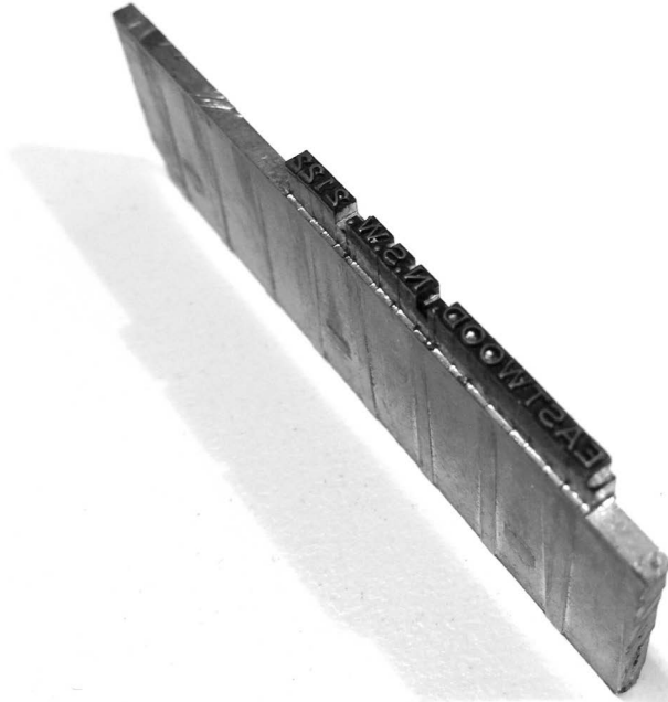
Fig. 69 Linotype slug, artefact courtesy of Ray Utick, photograph by the author.
