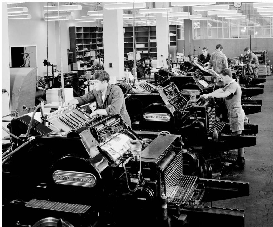
Fig. 56 Press-machinist John Wetherell works on a Heidelberg cylinder letterpress machine, 1965. Others pictured may be Dicky Carroll and Phillip Brook. Copyright of the Crown, reproduced with permission, courtesy of the Mitchell Library, State Library of New South Wales, Sydney. SLNSW call no. Government Printing Office 2 - 27294.
