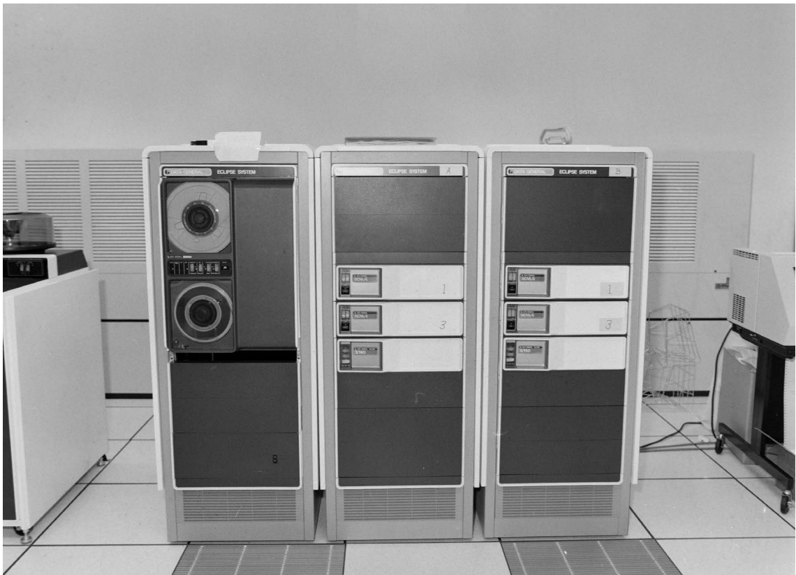
Fig. 72 The swiftly obsolescent Autologic MTU machines, 1984, part of the Penta typesetting system installed at the Government Printing Office. Copyright of the Crown, reproduced with permission, courtesy of the Mitchell Library, State Library of New South Wales, Sydney. SLNSW call no. PXA63391, Government Printing Office 4 – 29154.
